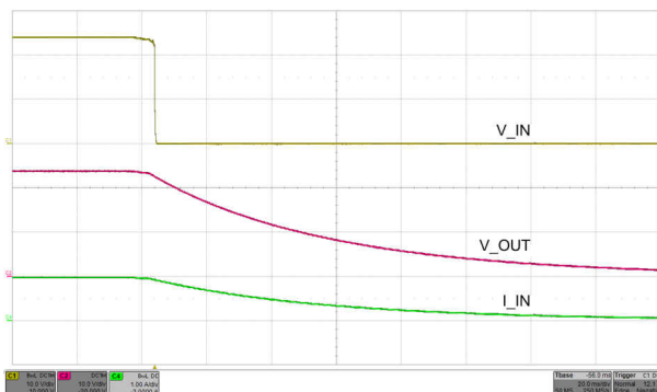
图 10-9. Power Fail With 24-Ω Load—Supports 1-A Load for 10-ms Power Fail
