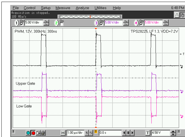
图 7-4. 12-V PWM Pulse at V_{DD} = 7.2 V
