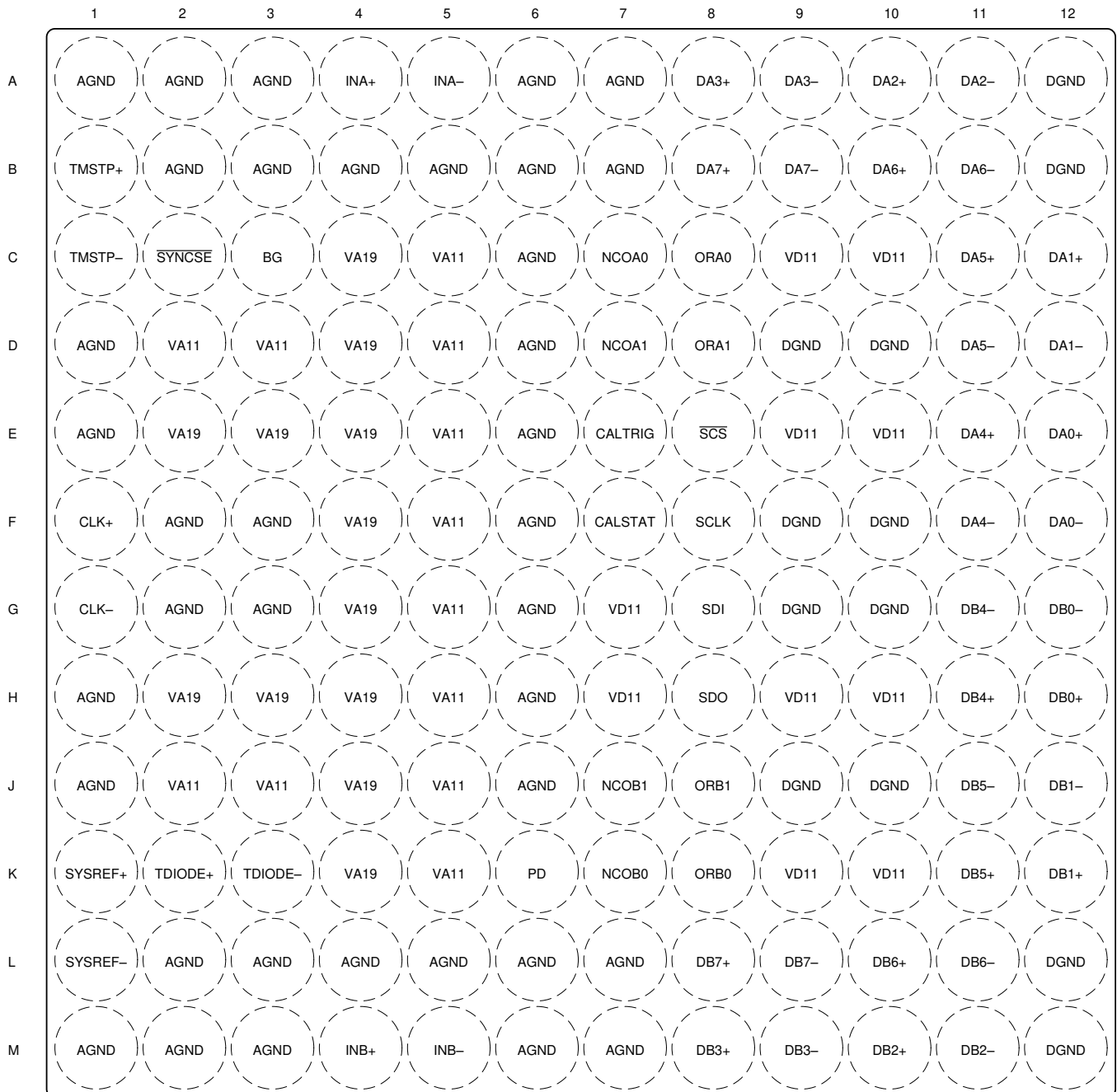
AAV Package 144-Ball Flip Chip BGA Top View
