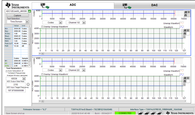
图 189. Idle-Channel Noise (No Input) for 2.5-GSPS, Dual-Channel Oscilloscope
