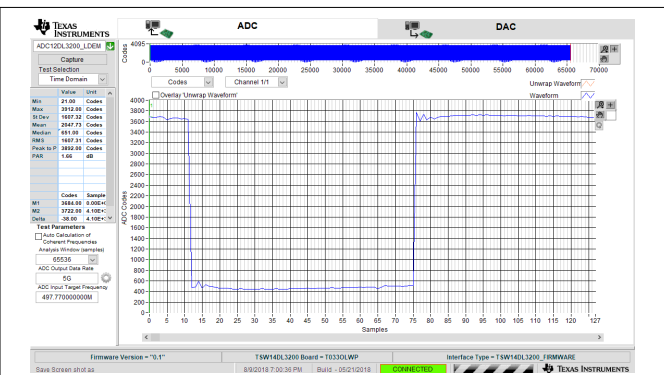
图 8-6. 40-MHz, Square-Wave Time Domain for 5-GSPS, Single-Channel Oscilloscope
