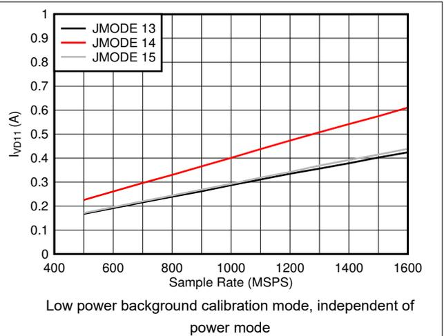
图 5-88. Quad Channel,  $I_{VD11}$  vs  $F_S$  and JMODE 13 - 15
