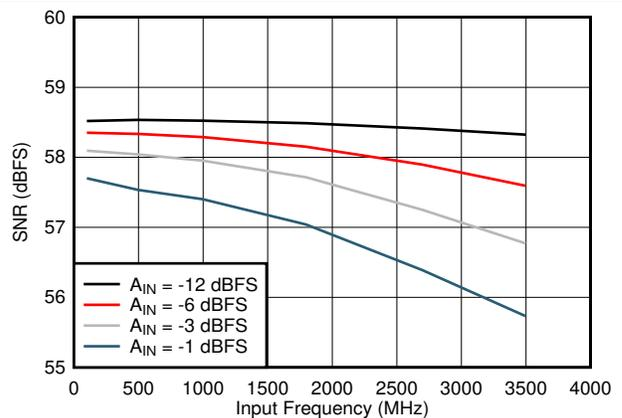
图 5-18. SNR vs Input Frequency
