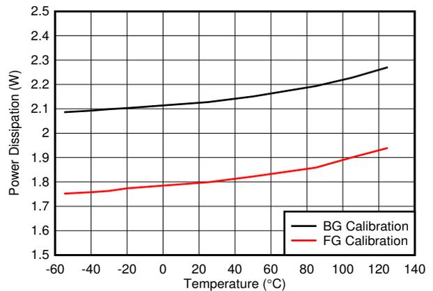
图 5-122. Dual Channel, Power Dissipation vs Temperature
