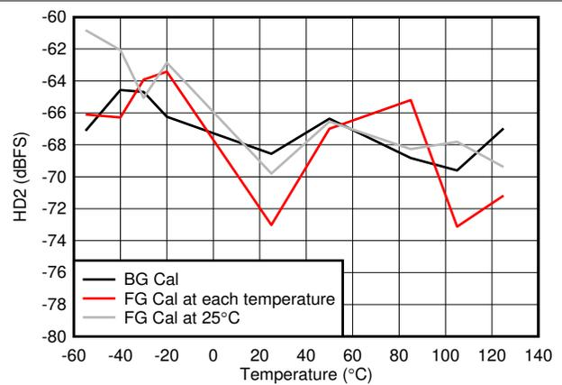
图 5-66. HD2 vs Temperature
