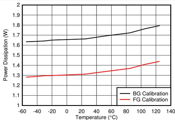
图 5-123. Single Channel, Power Dissipation vs Temperature
