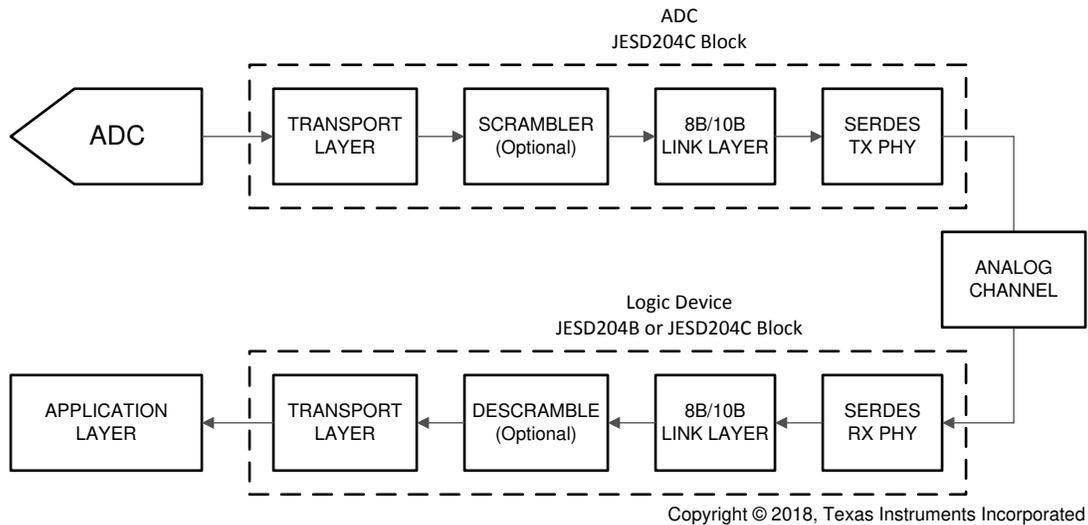
图 6-5. Simplified 8B/10B Encoded JESD204C Interface Diagram
