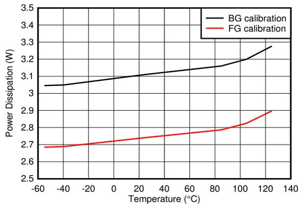
图 5-121. Quad Channel, Power Dissipation vs Temperature
