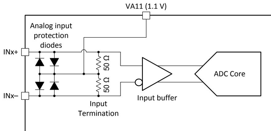
**图 6-2. Analog Input Internal Termination and Protection Diagram**
