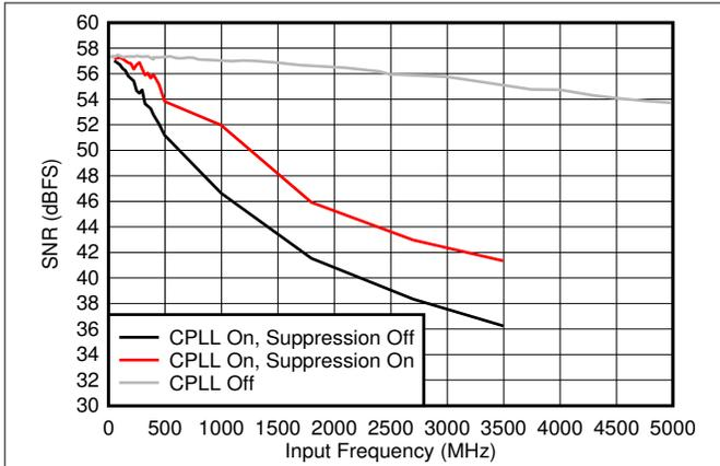
图 5-41. SNR vs  $F_{IN}$  and C-PLL modes
