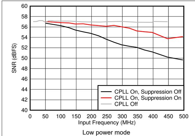
图 5-45. SNR vs  $F_{IN}$  and C-PLL modes
