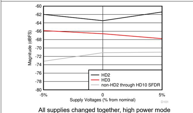
图 5-61. HD2, HD3 and Worst non-HD Spur vs Supply Voltage
