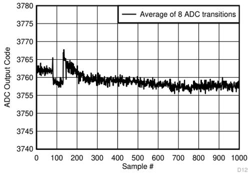
BG Calibration, input voltage offset ~ 90% of fullscale,
