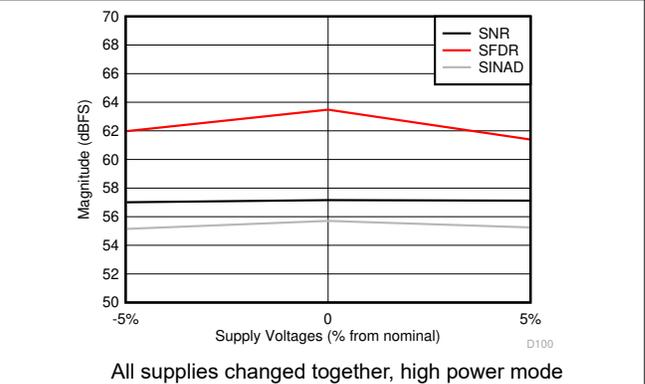
图 5-60. SNR, SFDR and SINAD vs Supply Voltage
