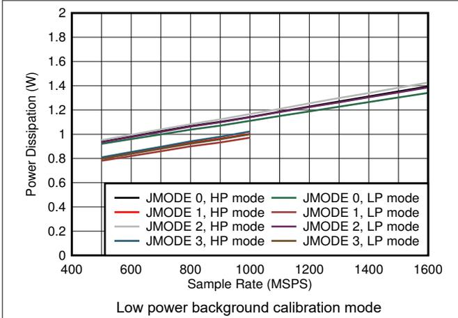
图 5-99. Single Channel, Power Dissipation vs  $F_S$  and JMODE 0
