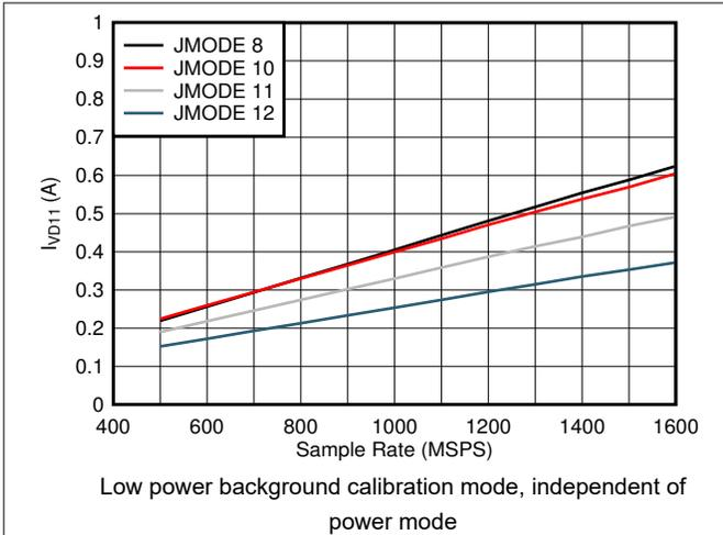
图 5-87. Quad Channel,  $I_{VD11}$  vs  $F_S$  and JMODE 8 - 12
