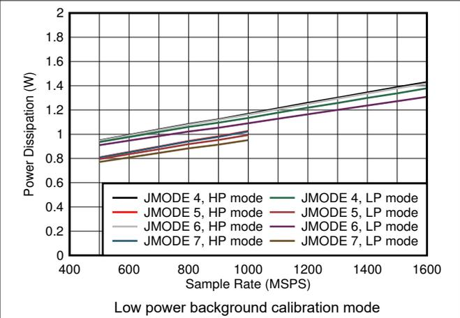
图 5-100. Single Channel, Power Dissipation vs  $F_S$  and JMODE 4
