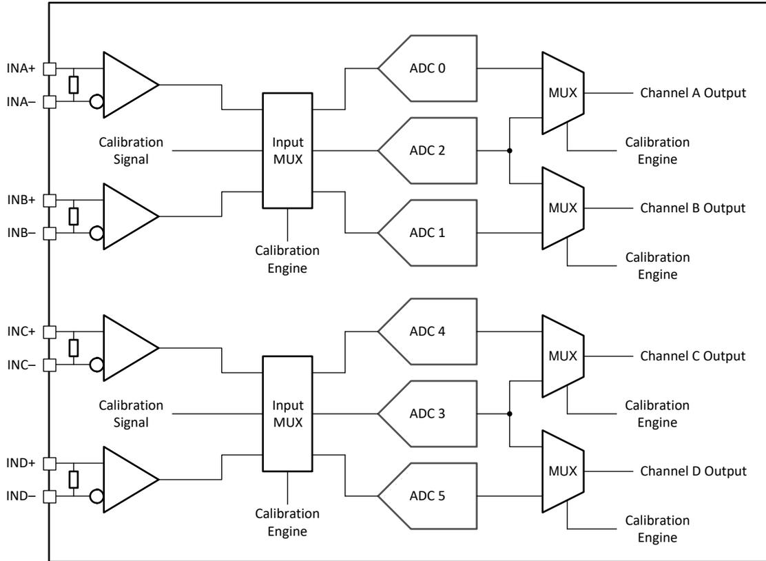
图 6-13. Quad Channel Calibration System Block Diagram
