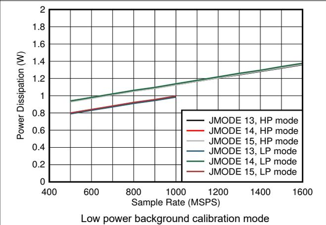
图 5-102. Single Channel, Power Dissipation vs  $F_S$  and JMODE
