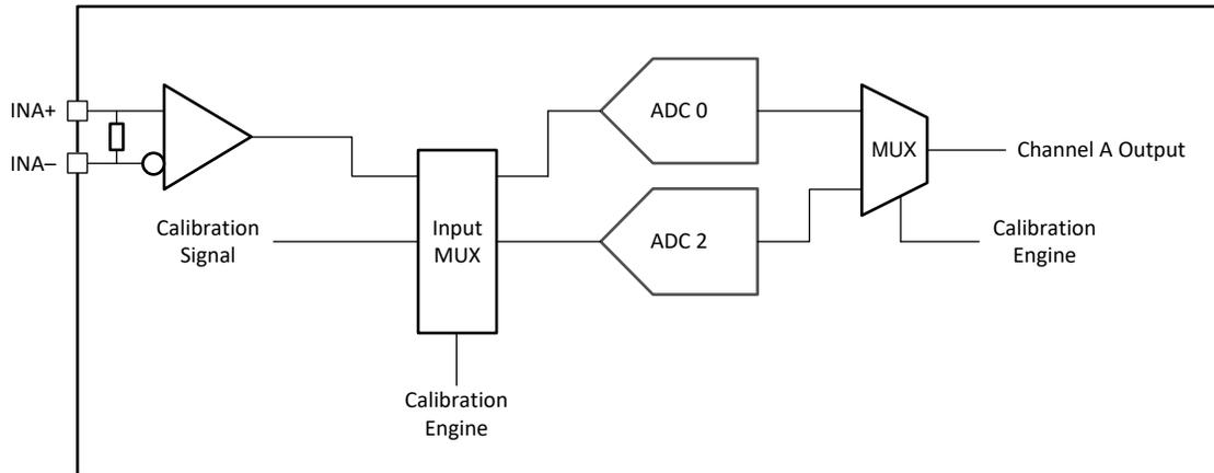
图 6-15. Single Channel Calibration System Block Diagram
