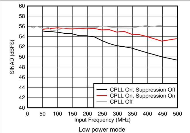
图 5-46. SINAD vs  $F_{IN}$  and C-PLL modes
