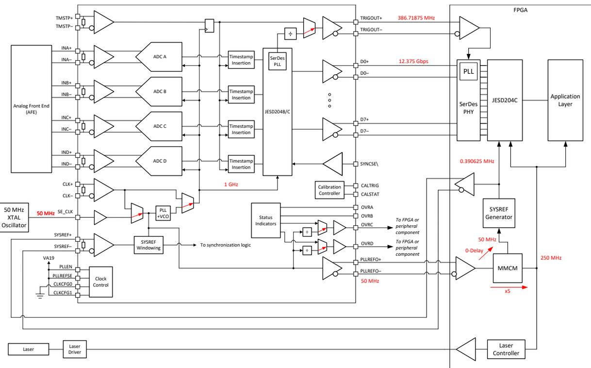
图 7-1. Typical Configuration for a LiDAR Digitizer
