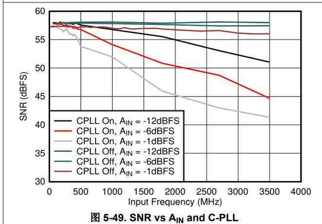
图 5-49. SNR vs  $A_{IN}$  and C-PLL
