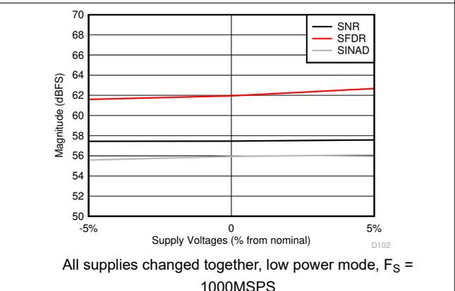
图 5-62. SNR, SFDR and SINAD vs Supply Voltages
