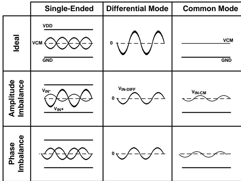
图 60. Differential Signal Waveform and Signal Imbalance
