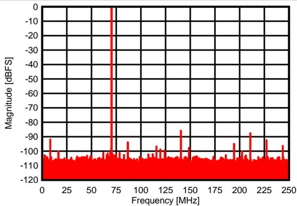
图 18. Output Spectrum, 1-Tone Test at 70 MHz
