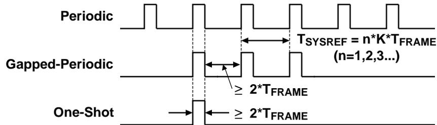
**图 73. SYSREF Signal Types (Single-Ended Representations)**
