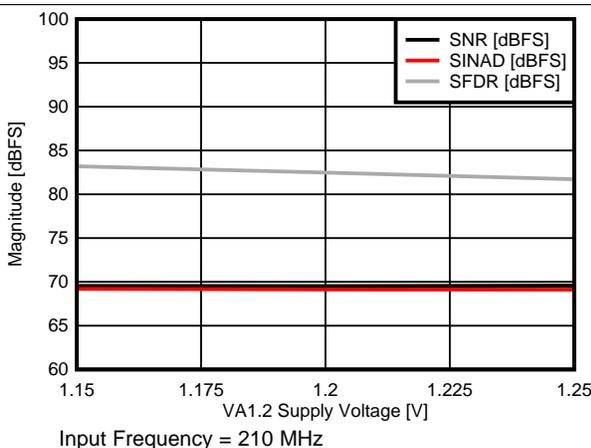
图 12. SNR, SINAD, SFDR vs VA1.2 Supply
