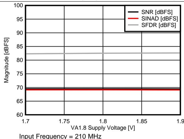
图 11. SNR, SINAD, SFDR vs VA1.8 Supply
