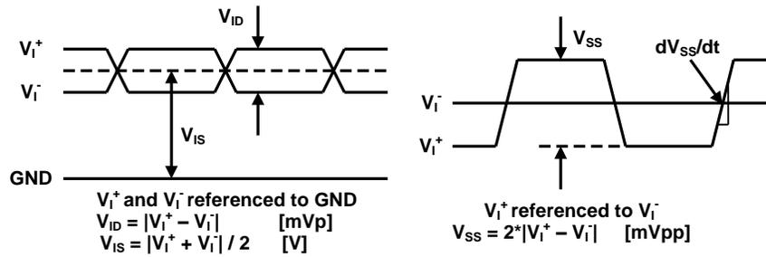
图 26. Electrical Level Diagram for Differential Input Signals
