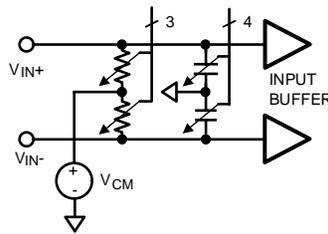
**图 30. Simplified Input Differential Balance Correction Circuit**
