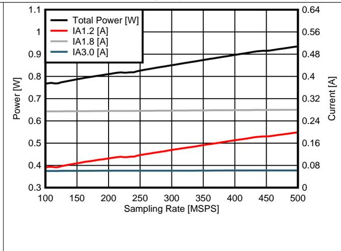
图 23. Supply Power and Current vs Sampling Rate
