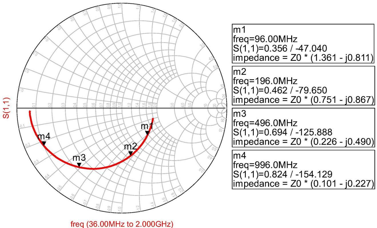
图 62. Differential 1-Port S-Parameter Measurement of the ADC Input (Sdd11, Z<sub>0</sub>=100 Ω)
