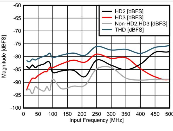
图 14. HD2, HD3, SPUR, THD vs Input Frequency
