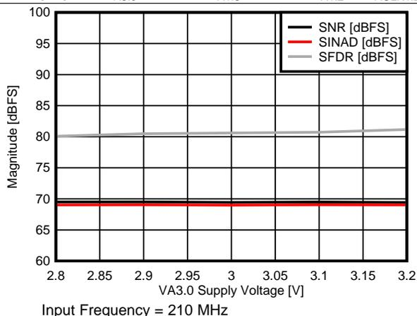
图 10. SNR, SINAD, SFDR vs VA3.0 Supply
