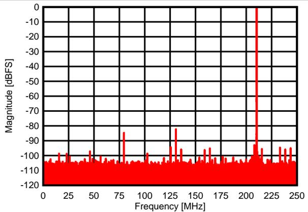
图 19. Output Spectrum, 1-Tone Test at 210 MHz
