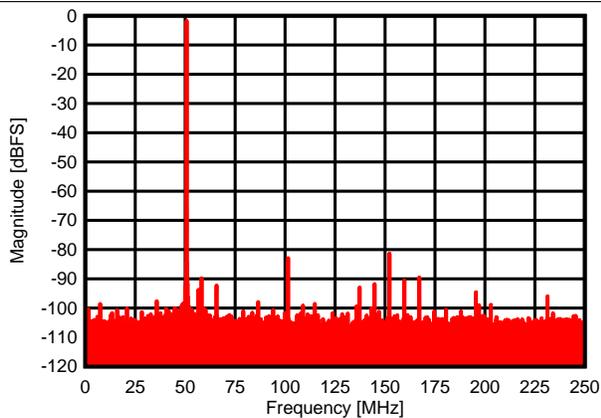
图 20. Output Spectrum, 1-Tone Test at 450 MHz
