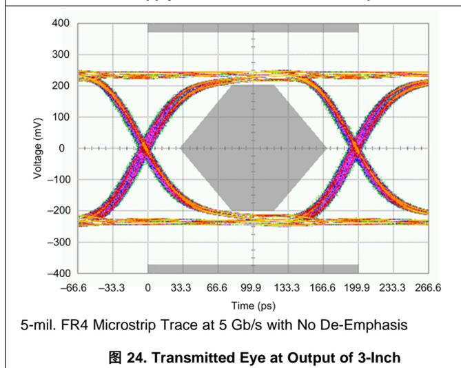
图 24. Transmitted Eye at Output of 3-Inch
