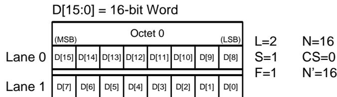
图 34. Transport Layer Definitions for the Supported-Lane Configurations
