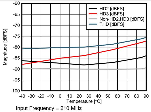
图 17. HD2, HD3, SPUR, THD vs Temperature
