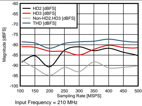
图 16. HD2, HD3, SPUR, THD vs Sampling Rate
