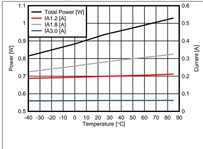
图 22. Supply Power and Current vs Temperature
