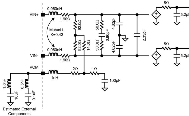
图 61. Simplified Analog Input Network Circuit Model
