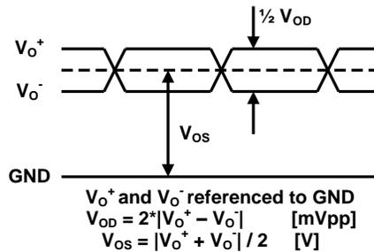
图 28. Electrical Level Diagram for Differential Output Signals
