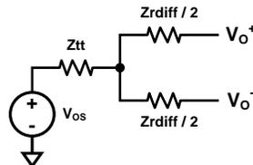
图 29. Electrical Circuit Diagram for Differential Output Signals
