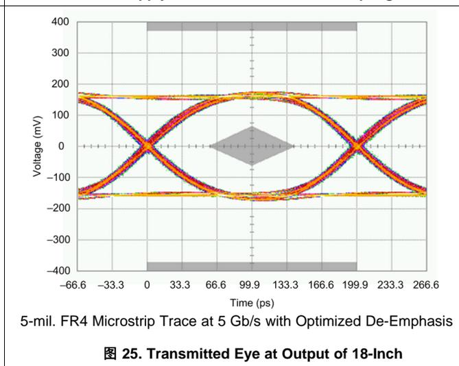
图 25. Transmitted Eye at Output of 18-Inch
