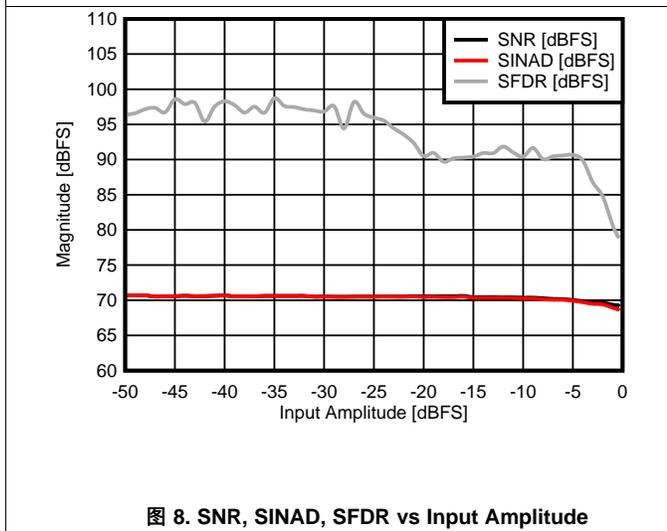
图 8. SNR, SINAD, SFDR vs Input Amplitude
