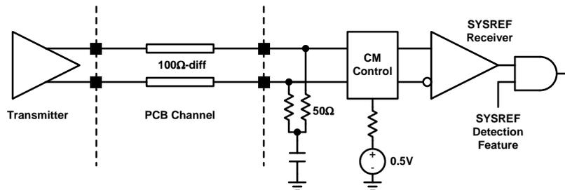
图 72. SYSREF Input Receiver and DC Coupled Interface
