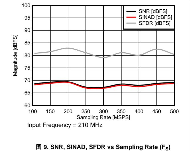
图 9. SNR, SINAD, SFDR vs Sampling Rate ( $F_s$ )
