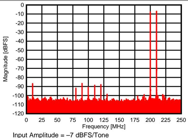
图 21. Output Spectrum, 2-Tone Test at 200 MHz and 210 MHz
