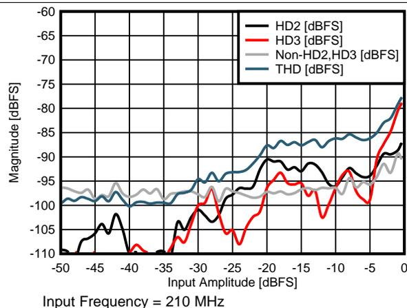
图 15. HD2, HD3, SPUR, THD vs Input Amplitude
