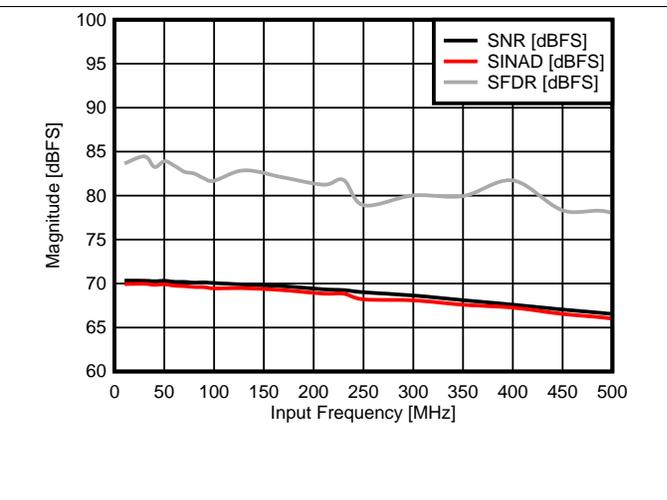
图 7. SNR, SINAD, SFDR vs Input Frequency
