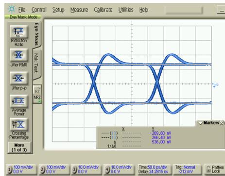
图 32. De-emphasis of the Differential Output Signal
