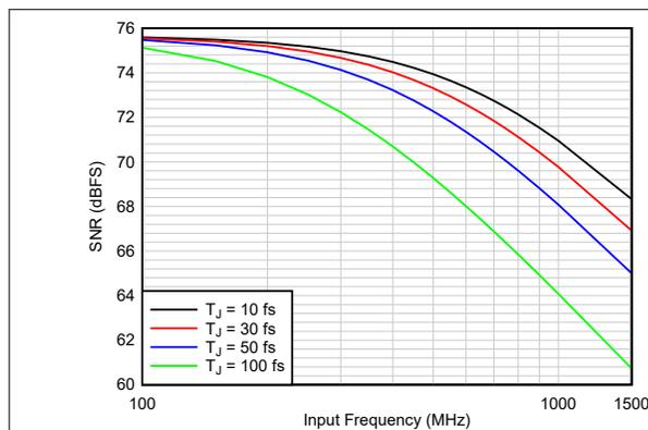
图 8-2. SNR 与  $T_{\text{jitter}}$  间的关系
