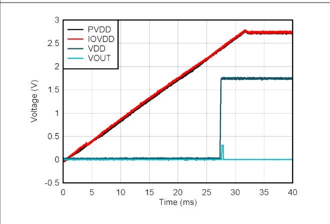
图 5-26. DAC 电源上电, PVDD = 2.7V
