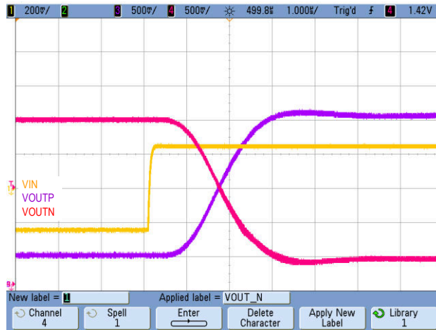
图 8-4. Step Response of the AMC1301
