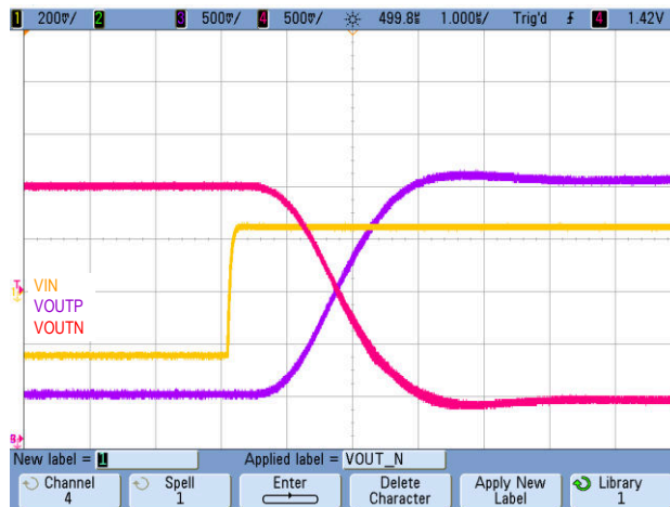
图 8-4. Step Response of the AMC1301
