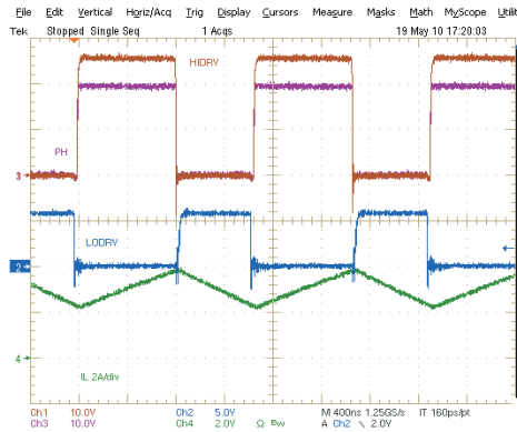
CH1: PHASE, 10V/div, CH2: LODRV, 5V/div, CH3: HIDRV, 10V/div, CH4: inductor current, 2A/div, 400ns/div
