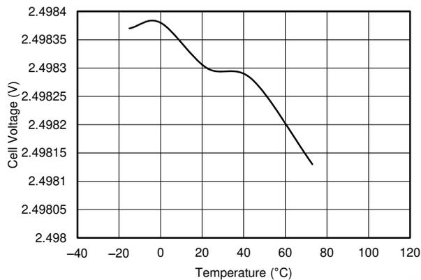
**图 7-14. V<sub>CELL</sub> Measurement at 2.5-V vs. Temperature**
