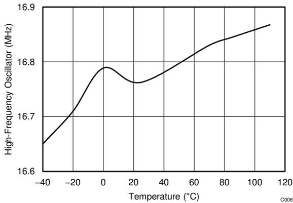
图 7-6. High-Frequency Oscillator vs. Temperature
