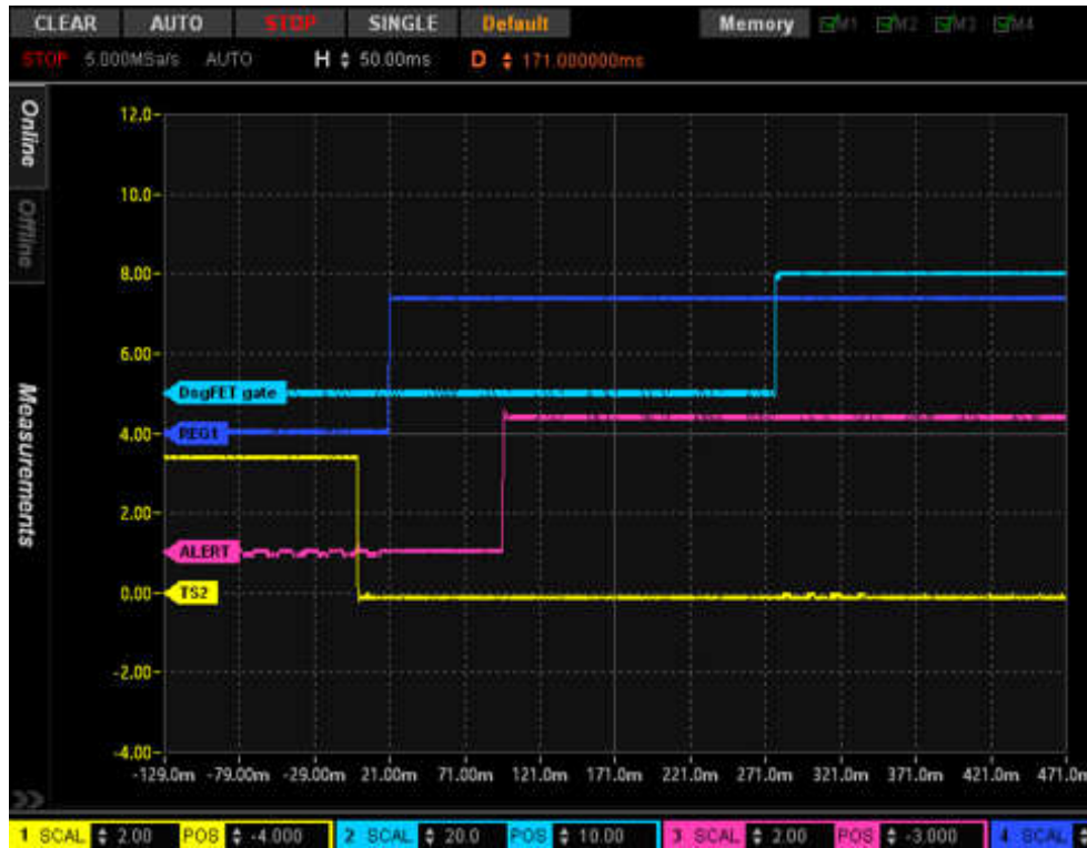
图 8-7. Startup Sequence Using [FASTADC] = 0 , with the [FULLSCAN] Flag Displayed on the ALERT Pin
