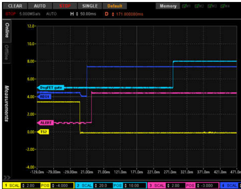
图 8-6. Startup Sequence Using [FASTADC] = 1 , with the [INITCOMP] Flag Displayed on the ALERT Pin
