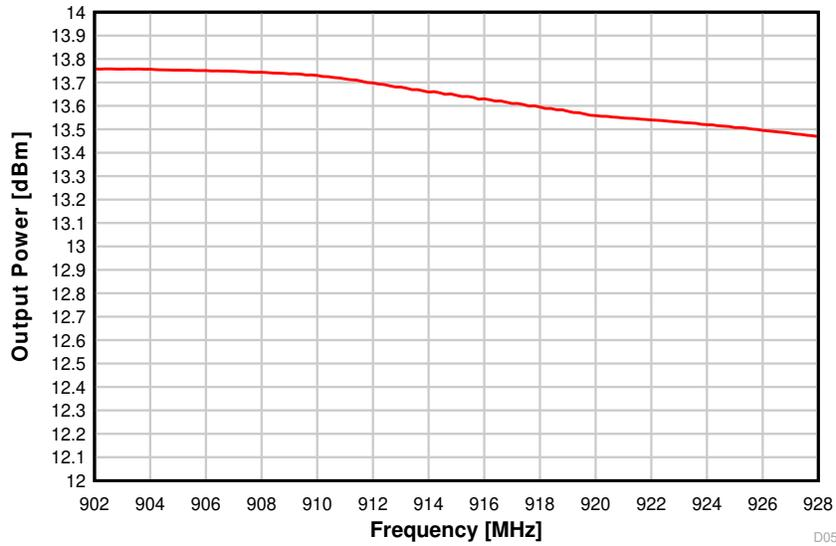
图 8-24. Output Power vs. Frequency (50 kbps, 915 MHz)
