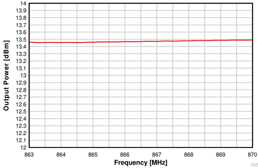
图 8-23. Output Power vs. Frequency (50 kbps, 868 MHz)
