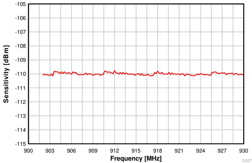
图 8-13. Sensitivity vs. Frequency (50 kbps, 915 MHz)
