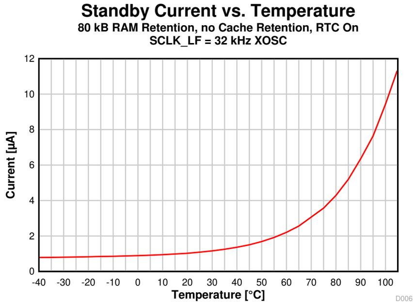
图 8-5. Standby Mode (MCU) Current vs. Temperature
