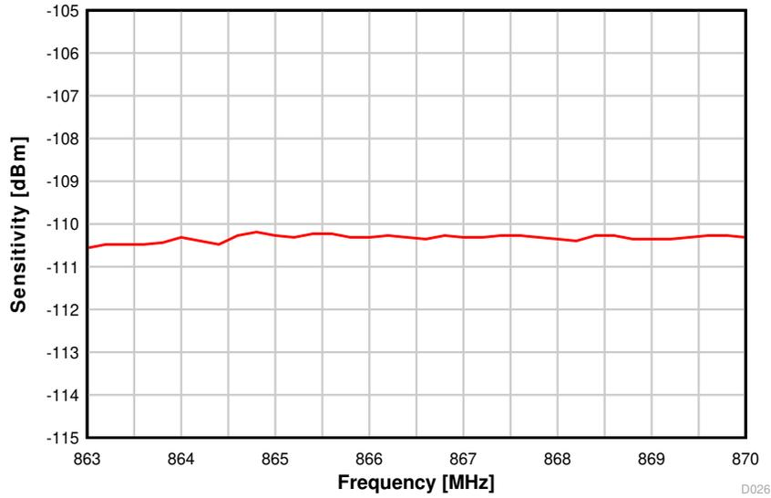
图 8-12. Sensitivity vs. Frequency (50 kbps, 868 MHz)
