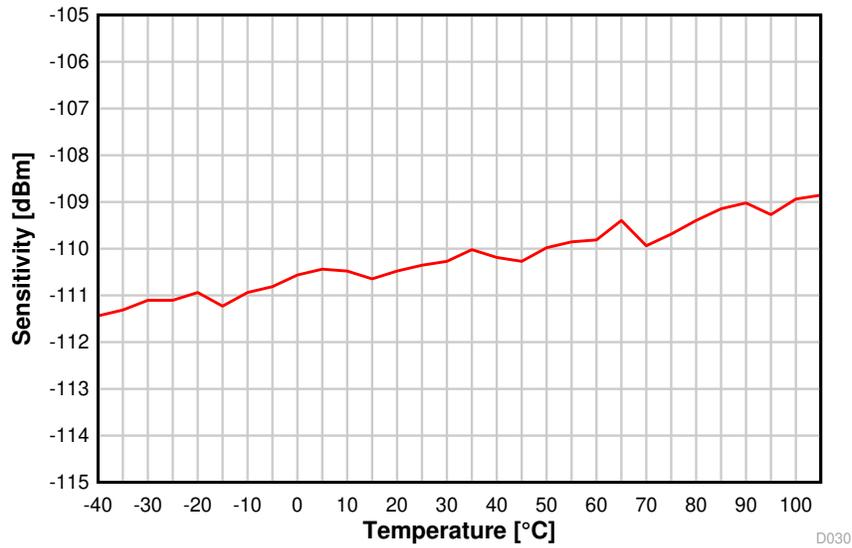
图 8-14. Sensitivity vs. Temperature (50 kbps, 868.3 MHz)
