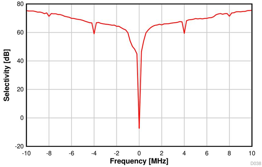
图 8-16. Selectivity vs. Frequency Offset (50 kbps, 868.3 MHz)
