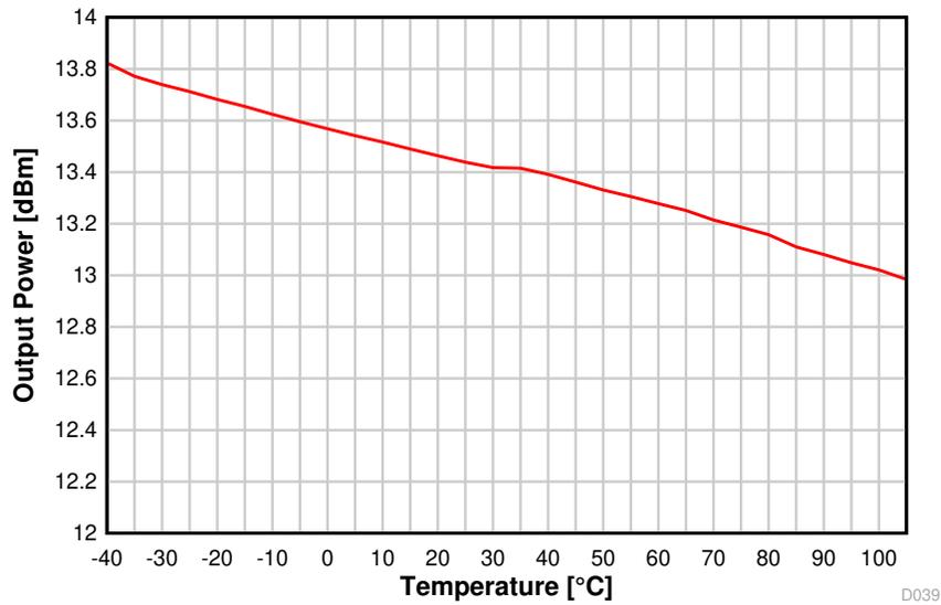
图 8-21. Output Power vs. Temperature (50 kbps, 868.3 MHz)
