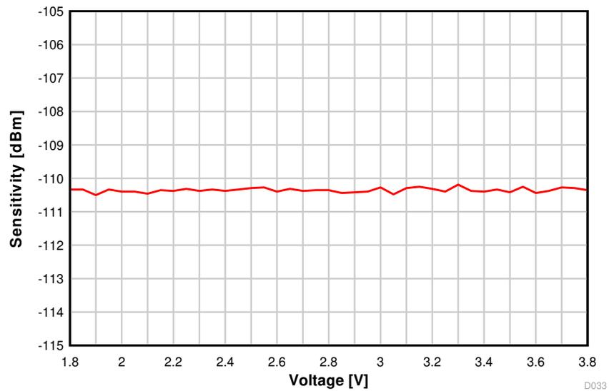
图 8-15. Sensitivity vs. Supply Voltage (VDDS) (50 kbps, 868.3 MHz)
