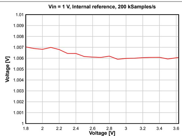
图 8-30. ADC Accuracy vs. Supply Voltage (VDD5)
