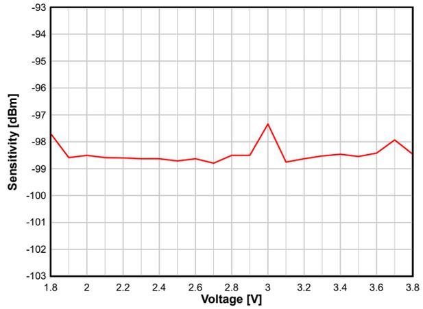
**图 8-18. Sensitivity vs. Supply Voltage (VDDS) (250 kbps, 2.44 GHz)**
