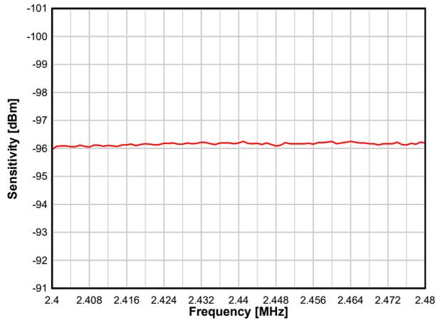
**图 8-12. Sensitivity vs. Frequency (BLE 1 Mbps, 2.44 GHz)**
