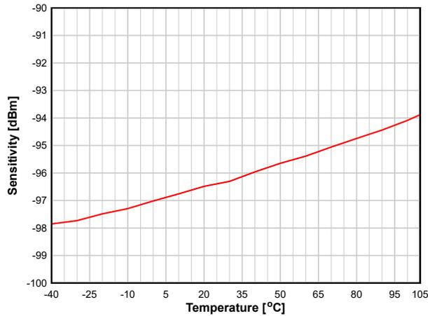
**图 8-14. Sensitivity vs. Temperature (BLE 1 Mbps, 2.44 GHz)**
