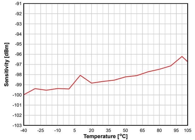
**图 8-15. Sensitivity vs. Temperature (250 kbps, 2.44 GHz)**
