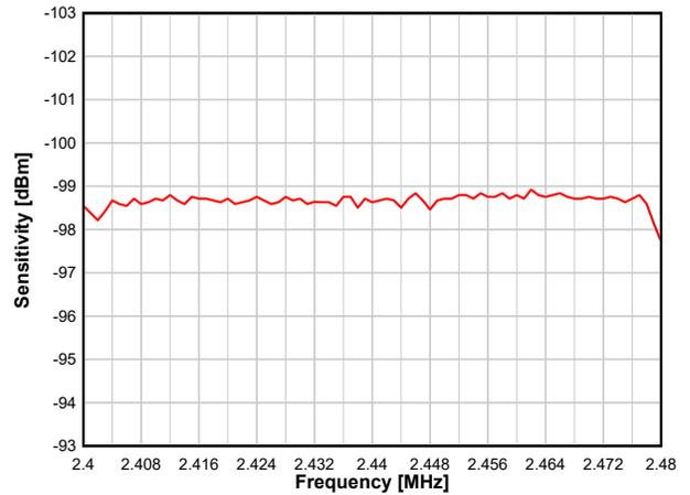
**图 8-13. Sensitivity vs. Frequency (250 kbps, 2.44 GHz)**
