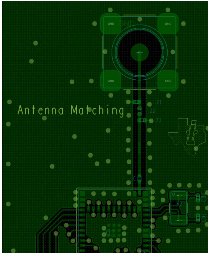
图 10-5. Module Layout Guidelines with External Antenna
