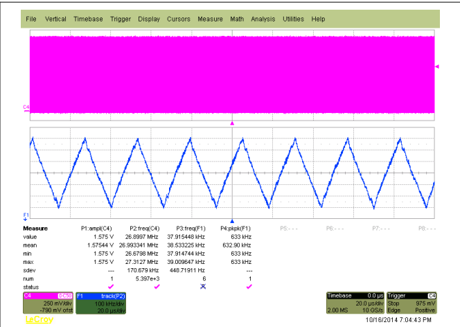
图 9-7. f_{out} = 27\text{MHz} , VCO frequency > 175MHz, SSC (1%, center)
