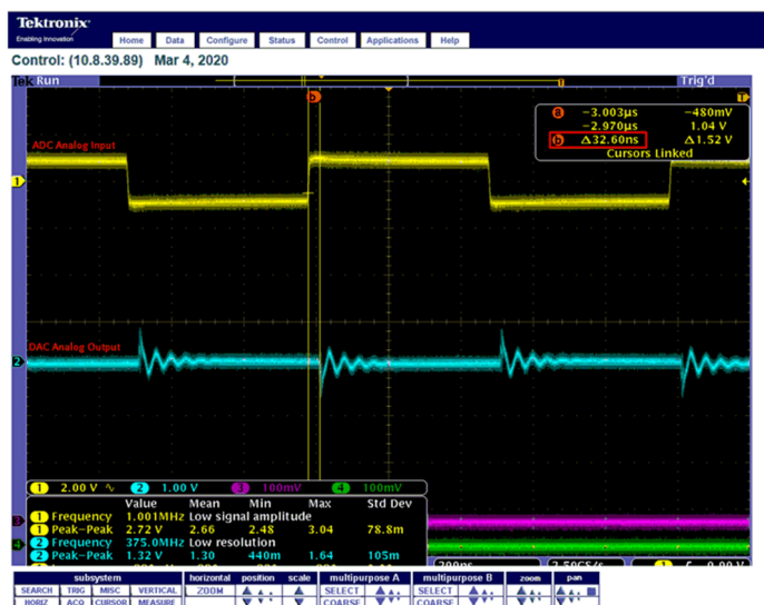
图 8-4. ADC Input to DAC Output Time for MSB loopback test.
