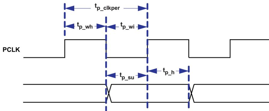
Figure 3. Parallel and BT.656 I/F General Timing
