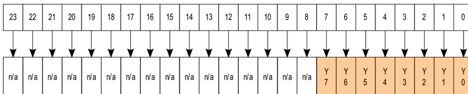
PDATA(7:0) of the Input Pixel data bus
