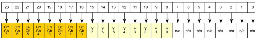
PDATA(23:0) of the Input Pixel data bus
