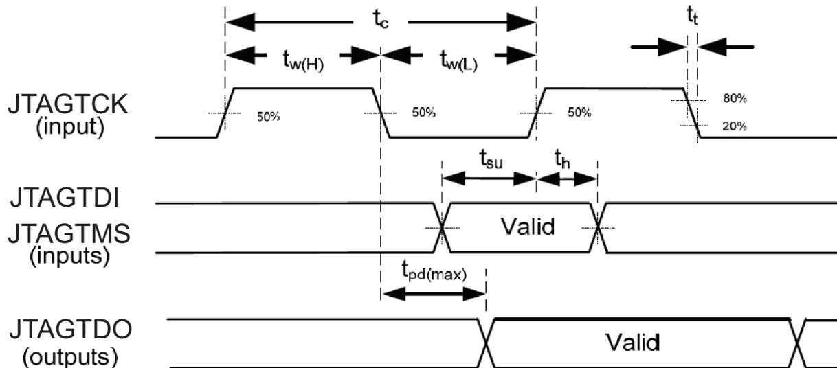
Figure 6. Boundary Scan Timing
