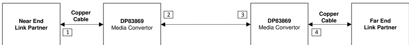
图 7-12. Link Loss Pass-Through
