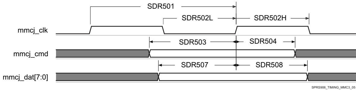
图 7-91. MMC/SD/SDIOj in - High Speed SDR50 - Receiver Mode
