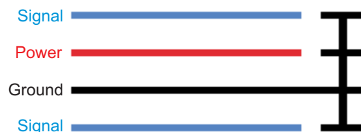
图 8-13. Guard Ring Routing
