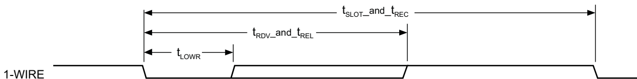
图 7-30. 1-Wire—Read Bit (Data)
