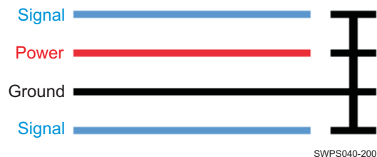
图 7-19. Guard Ring Routing
