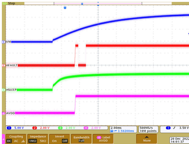
图 9-2. Device Power up with VM (VM, nFAULT, nSLEEP, AVDD)
