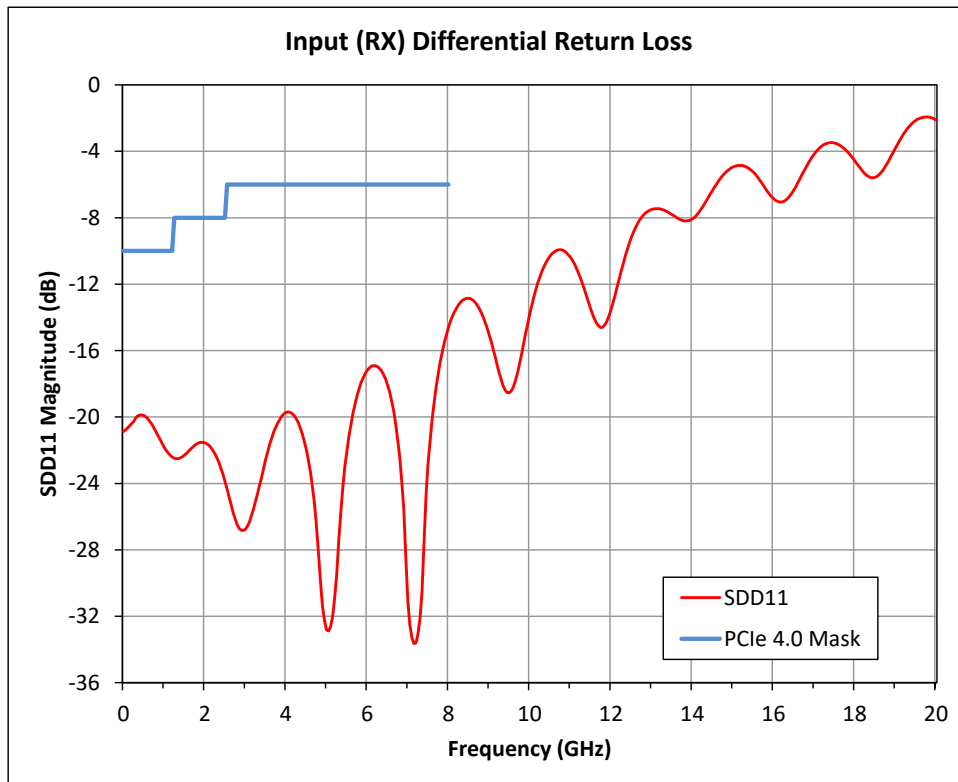
图 6-3. Typical RX Differential Return Loss
