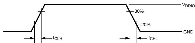
Figure 3. LVCMOS Transition Times
