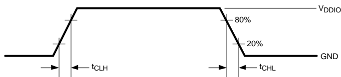
Figure 3. LVCMOS Transition Times
