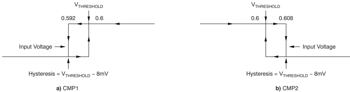
Figure 6-1. Comparator Hysteresis
