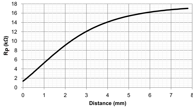
Figure 51. Example R_P vs. Distance with a 14-mm PCB Coil and 2mm Thick Stainless Steel Target
