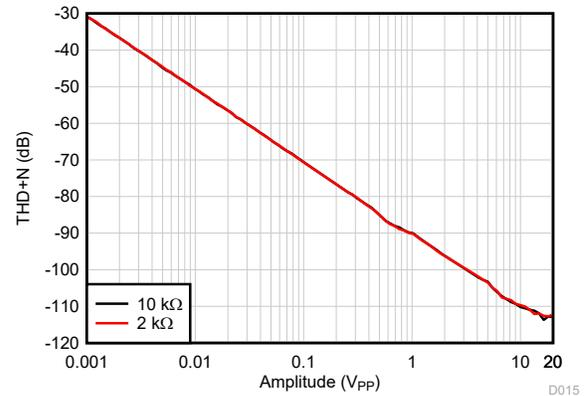
$G = 1$ ,  $f = 1\text{kHz}$ ,  $\text{BW} = 80\text{kHz}$ ,
