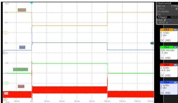
图 9-24. Average Output Current Limit ( $V_{(VIN)} = 12V$ ,
