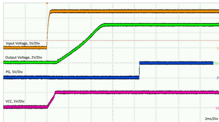
图 4. Typical Start-up Behavior V_{IN} = 12\text{ V} , V_{OUT} = 5\text{ V} , I_{OUT} = 4\text{ A}
