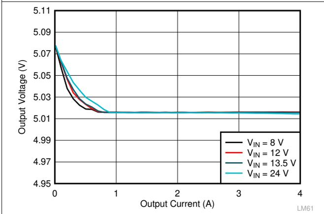
图 10-15. LM61440-Q1 Load and Line Regulation
