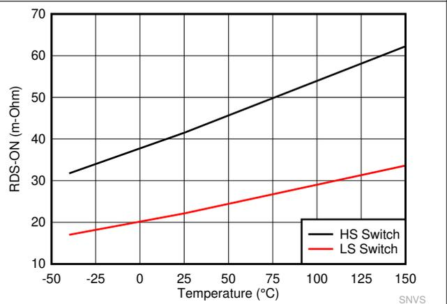
图 8-6. High-side and Low-side Switches  $R_{DS\_ON}$
