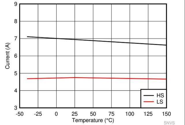
图 8-4. LM61440-Q1 High-side and Low-side Current Limits
