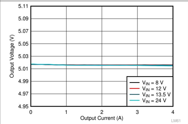
图 10-16. LM61440-Q1 Load and Line Regulation
