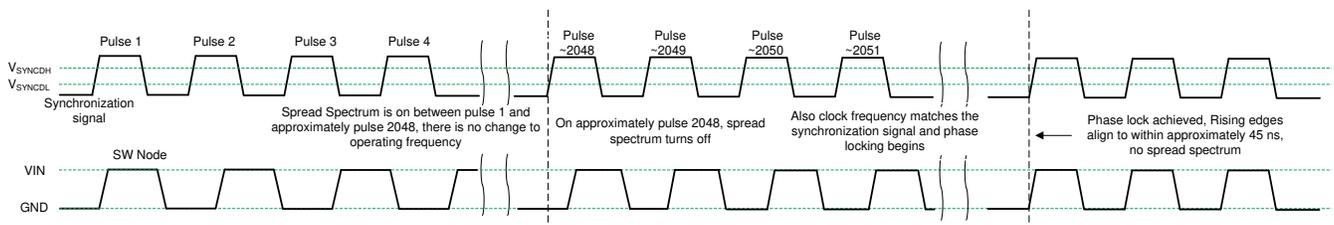
Pulses four and synchronization signal is detected. After the pulse, approximately 2048 ready to synchronize and frequency is adjusted using a glitch free technique. Later, phase is locked.
