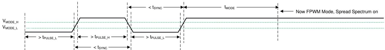
图 8-11. Transition from SYNC Mode to FPWM Mode
