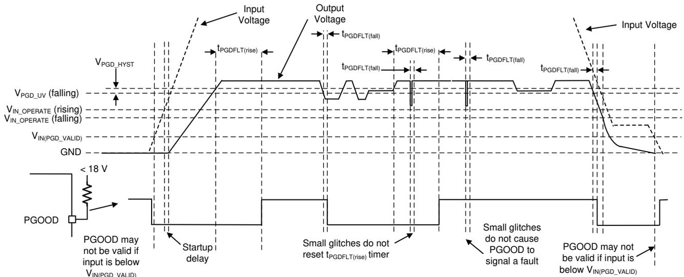
图 8-13. PGOOD Timing Diagram (Excludes OV Events)
