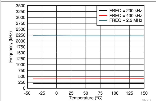
图 7-5. Switching Frequency Set by SYNC
