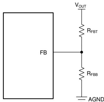
图 8-17. Setting Output Voltage of Adjustable Versions
