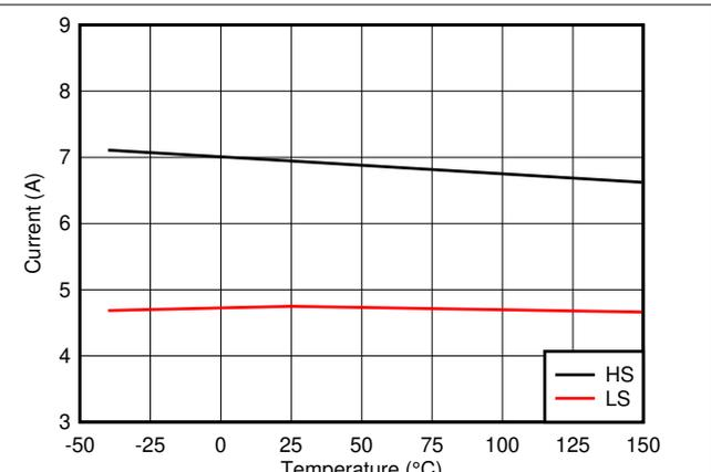
图 7-4. LM62435-Q1 High-side and Low-side Current Limits
