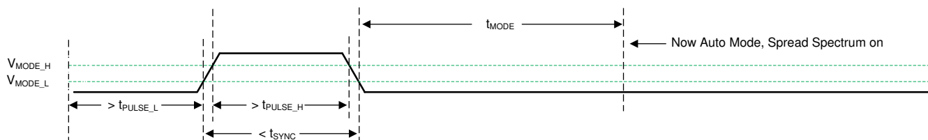
图 9-10. Transition from SYNC Mode to Auto Mode
