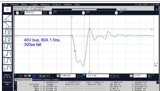
图 14. V_{DS} for 1.5 ns Pulse With 40V of Bus Voltage
