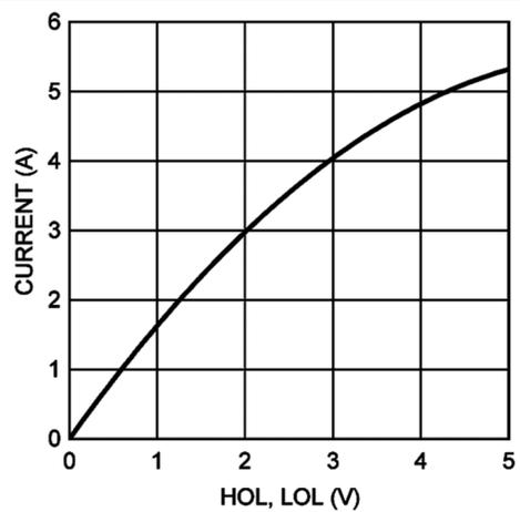
图 6-3. Peak Sink Current vs Output Voltage
