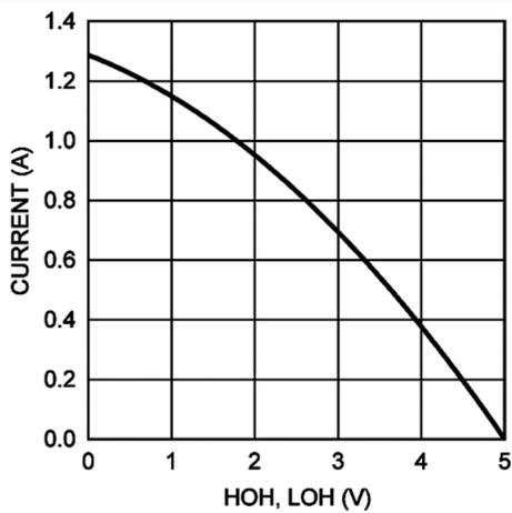
图 6-2. Peak Source Current vs Output Voltage
