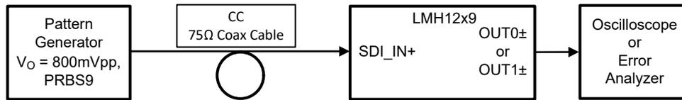
图 7-4. LMH12x9 PCB 输出 (OUT0 $\pm$ 、OUT1 $\pm$ ) 的测试设置
