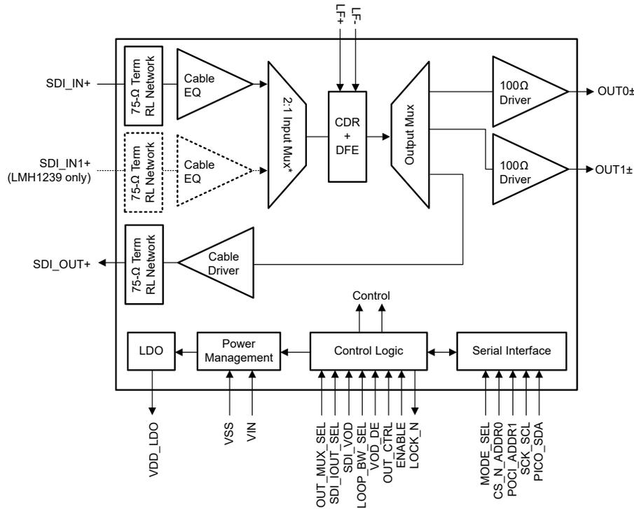
\*2:1 Input mux is only applicable with the LMH1239 variant. For LMH1229, SDI\_IN+ data path is routed directly to the CDR.
