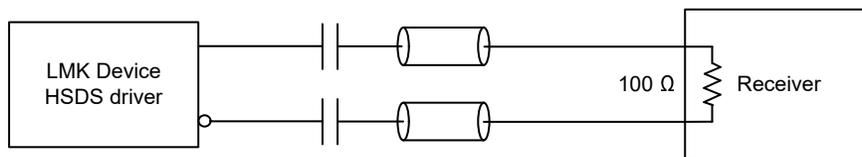
图 8-25. AC-Coupled HSDS Output Termination Method 1
