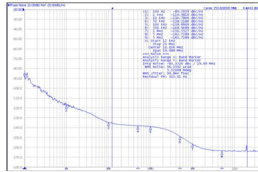
Jitter = 100 fs RMS (12 kHz to 20 MHz)
