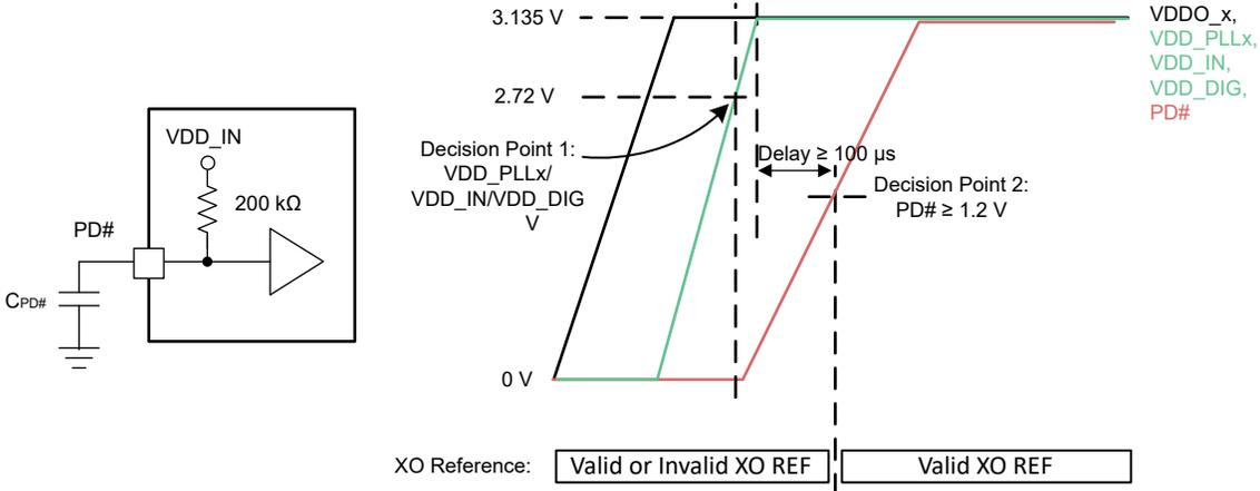
9-2. A capacitor from the PD# pin to GND can be used to form an RC time constant with the internal pullup resistor. This RC time constant can be designed to delay the low-to-high transition of PD# until all the core supplies have ramped above 3.135 V. TI recommends to ramp up VDDO supply pins before VDD supply pins.
