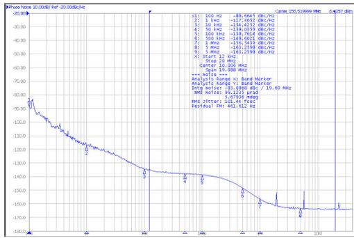
Jitter = 101 fs RMS (12 kHz to 20 MHz)
