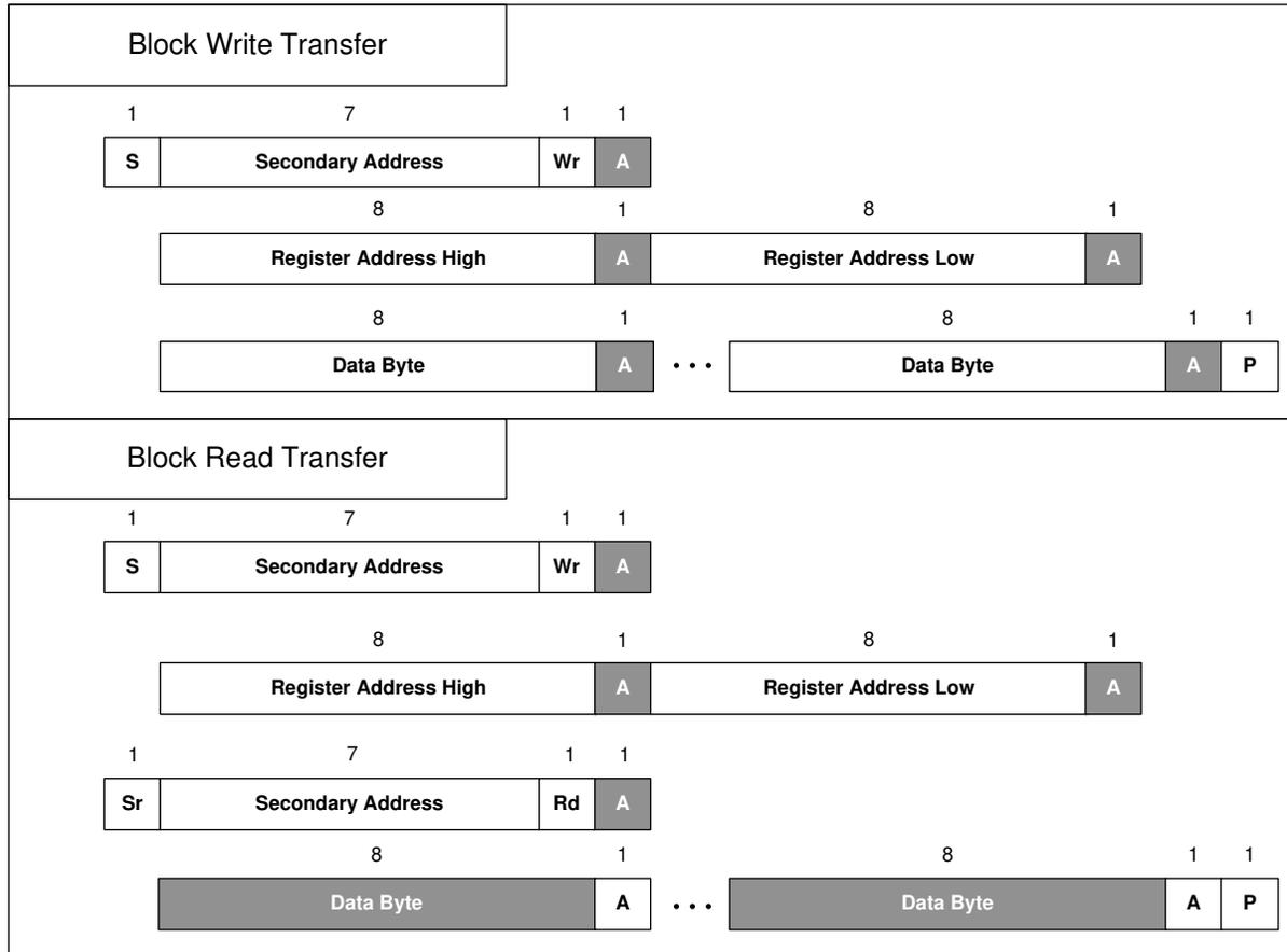
图 8-41. I<sup>2</sup>C Block Register Transfers
