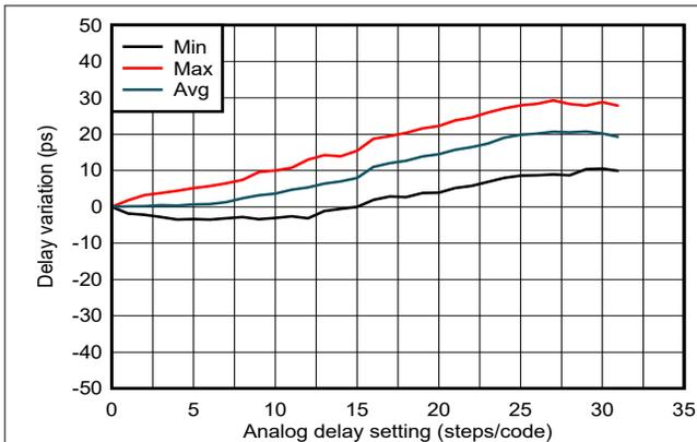
图 6-8. SYSREF/1-PPS Delay Linearity vs Analog Delay Code 2
