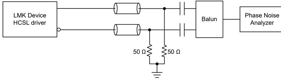
图 7-8. HCSL Output Time Domain Test Configuration
