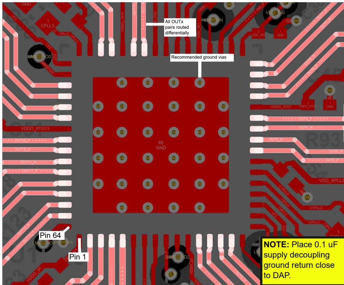
图 9-18. PCB Layout Example for LMK5B33216, Top Layer
