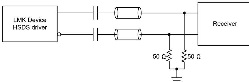
图 8-26. AC-Coupled HSDS Output Termination Method 2
