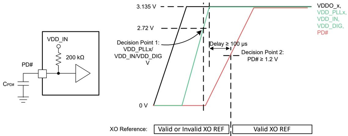
**图 9-2. Recommendation for Power Up From Split-Supply Rails**
