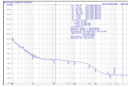
Jitter = 230 fs RMS (12 kHz to 20 MHz)
