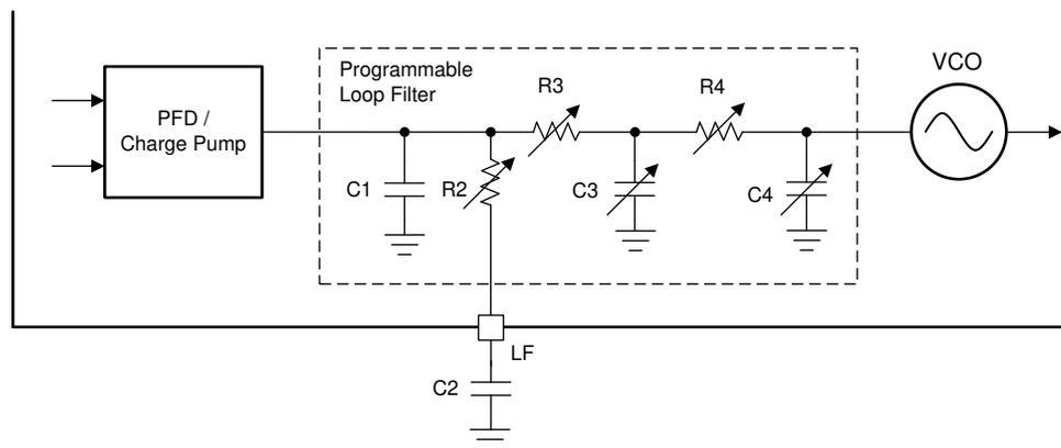
**图 8-22. Loop Filter Structure of Each APLL**
