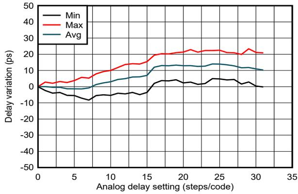
图 6-10. SYSREF/1-PPS Delay Linearity vs Analog Delay Code 4
