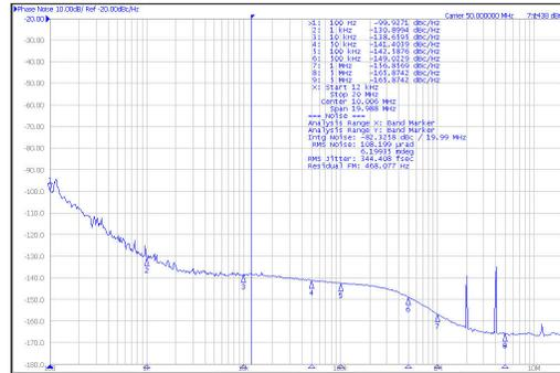
Jitter = 345 fs RMS (12 kHz to 20 MHz)
