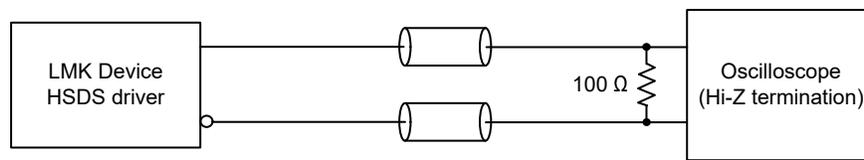
图 7-5. HSDS Output Time Domain Test Configuration
