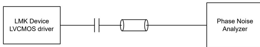
图 7-4. LVC MOS Output Phase Domain Test Configuration
