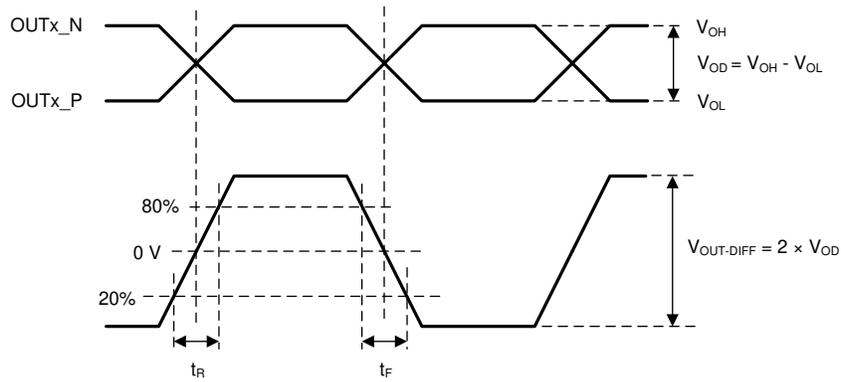
图 6-5. Differential Output Voltage and Rise/Fall Time
