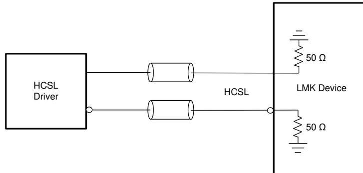
图 8-13. HCSL (Load Terminated) to Reference (INx)
