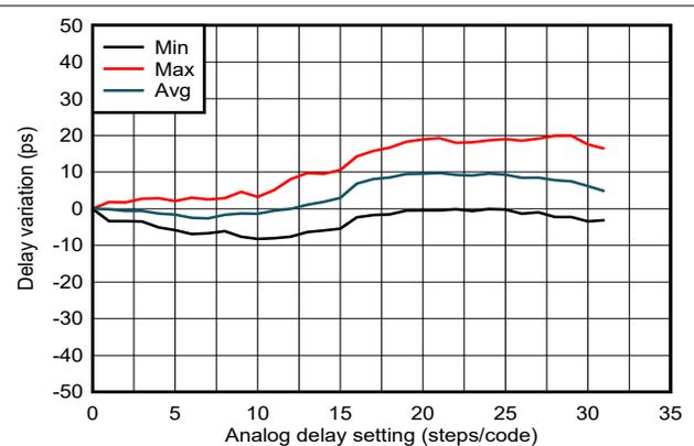
图 6-9. SYSREF/1-PPS Delay Linearity vs Analog Delay Code 3
