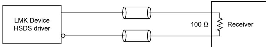
图 8-24. DC-Coupled HSDS Output Termination
