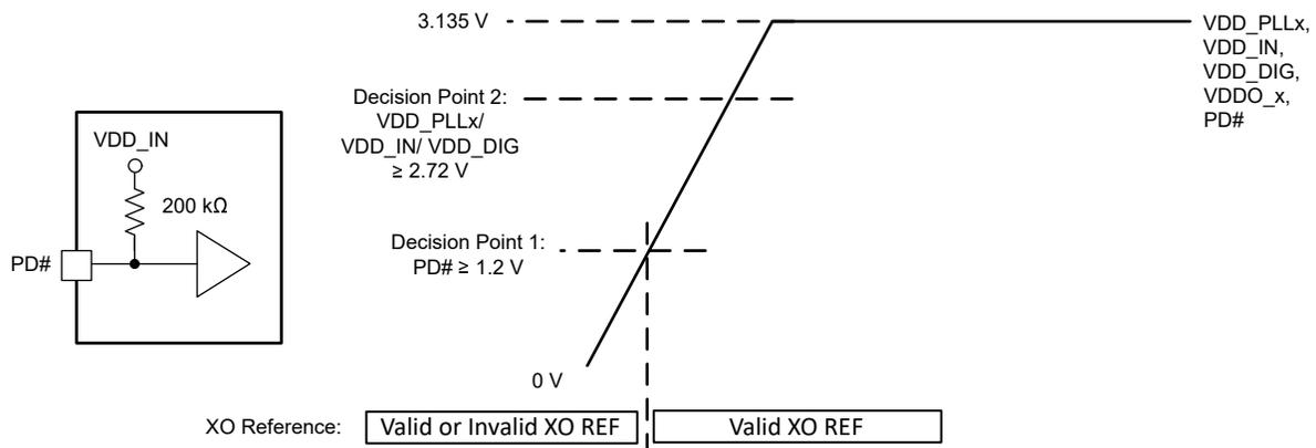
图 9-1. Recommendation for Power Up From a Single-Supply Rail
