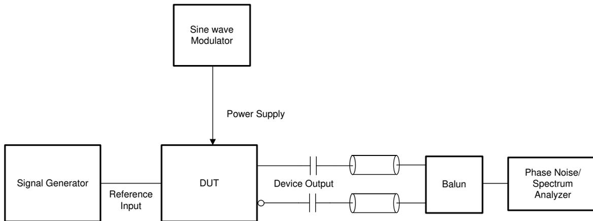
Single-side band spur level measured in dBc with a known noise amplitude and frequency injected onto the device power supply.
