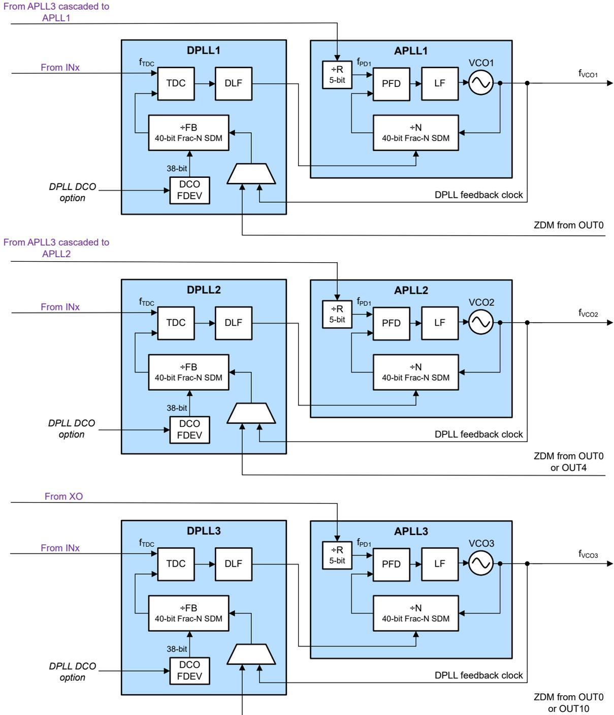
图 8-5. APLL Cascaded With DPLLs Enabled Example
