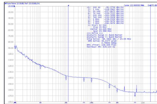
Jitter = 109 fs RMS (12 kHz to 20 MHz)
