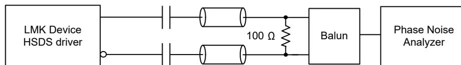
图 7-6. HSDS Output Phase Domain Test Configuration
