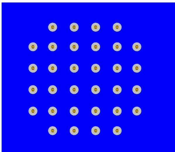
图 9-19. PCB Layout Example for LMK5B33216, Bottom Layer
