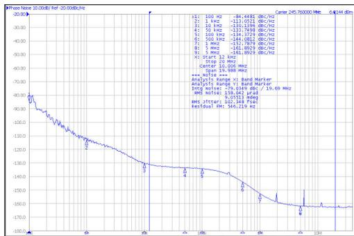
Jitter = 102 fs RMS (12 kHz to 20 MHz)
