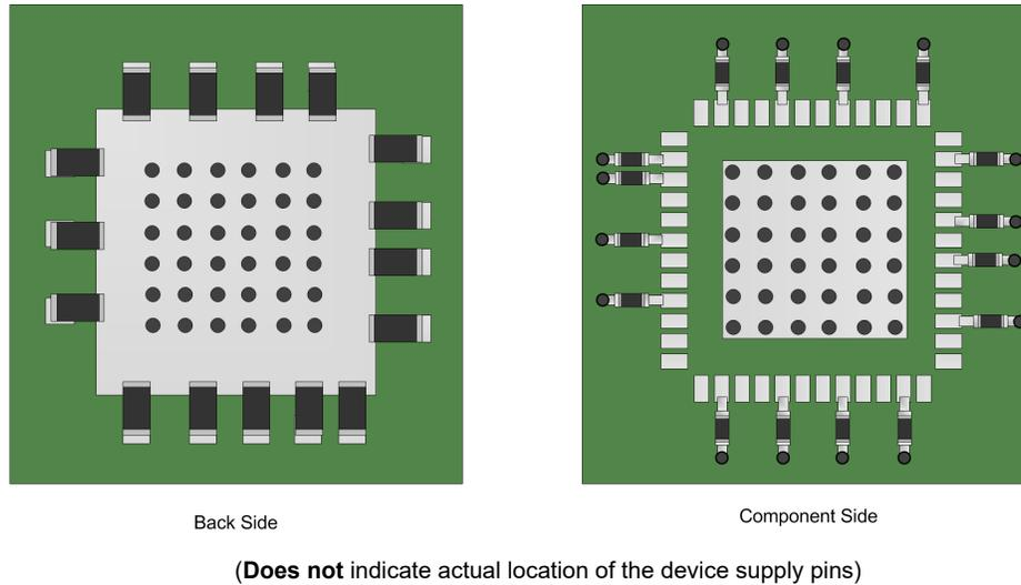
**图 9-17. Generalized Placement of Power Supply Bypass Capacitors**
