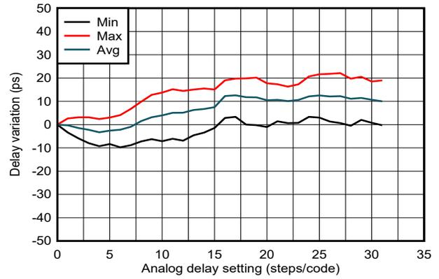
图 6-11. SYSREF/1-PPS Delay Linearity vs Analog Delay Code 5
