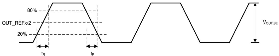
图 6-6. Single-Ended Output Voltage and Rise/Fall Time
