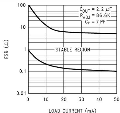
图 6-42. 2.2-  $\mu\text{F}$  ESR Curves for Legacy Chip
