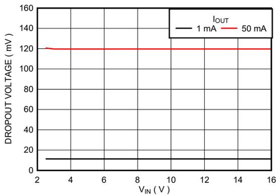
图 6-5. Dropout Voltage vs  $V_{IN}$  for New Chip
