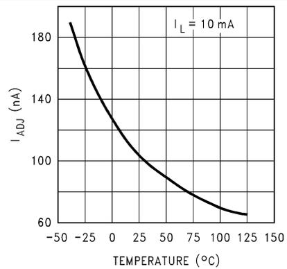
图 6-30. ADJ Pin Bias Current vs Temperature for Legacy Chip
