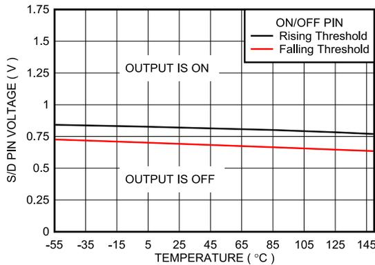
图 6-33. ON/OFF Threshold vs Temperature for New Chip
