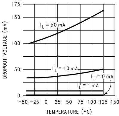
图 6-7. Dropout Voltage vs Temperature for Legacy Chip
