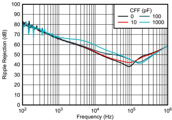
$V_{IN} = 4.3\text{ V}$ ,  $V_{OUT} = 3.3\text{ V}$ ,  $I_{OUT} = 50\text{ mA}$ ,  $C_{OUT} = 2.2\ \mu\text{F}$
