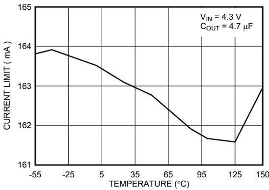
图 6-27. Short-Circuit Current vs Temperature for New Chip
