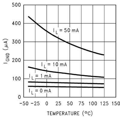
图 6-15. Ground-Pin Current vs Temperature for Legacy Chip
