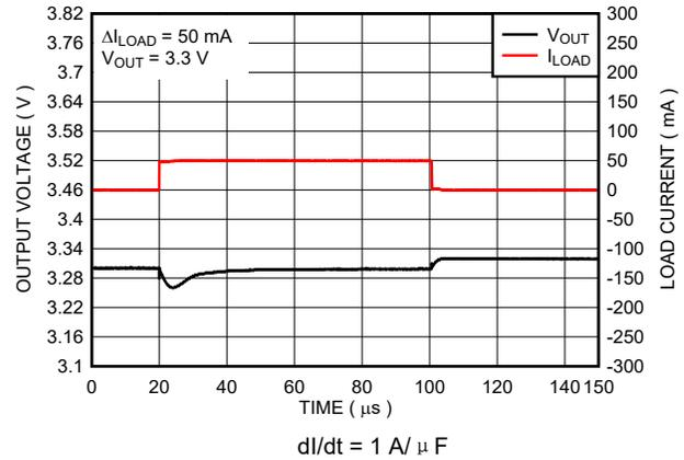
图 8-4. Load Transient Response for New Chip
