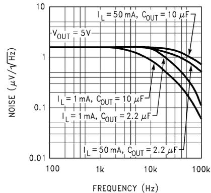
图 6-34. Output Noise Density for Legacy Chip
