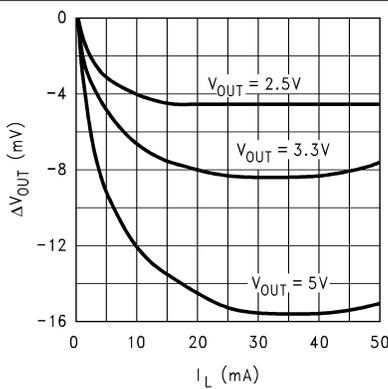
图 6-11. Output Regulation vs Load Current for Legacy Chip
