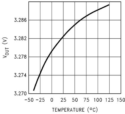
图 6-1. Output Voltage vs Temperature for Legacy Chip
