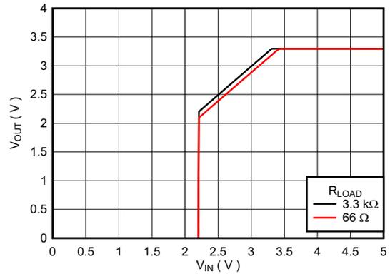
图 6-4. Output Voltage vs  $V_{IN}$  for New Chip
