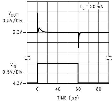
图 8-5. Line Transient Response for Legacy Chip
