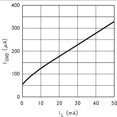
图 6-17. Ground Pin Current vs Load Current for Legacy Chip
