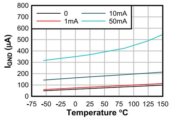
图 6-16. Ground-Pin Current vs Temperature for New Chip
