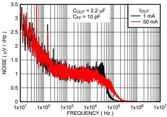
$V_{IN} = 4.3\text{ V}$ ,  $V_{OUT} = 3.3\text{ V}$ ,  $C_{OUT} = 2.2\ \mu\text{F}$ ,  $C_{FF} = 10\text{ pF}$
