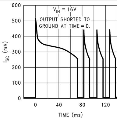
图 6-23. Short-Circuit Current vs Time for Legacy Chip
