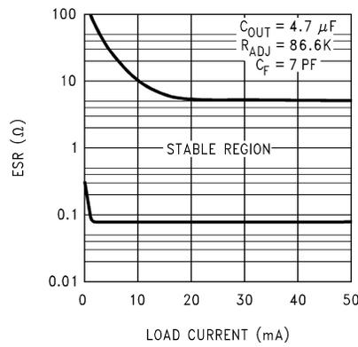
图 6-43. 4.7-  $\mu\text{F}$  ESR Curves for Legacy Chip
