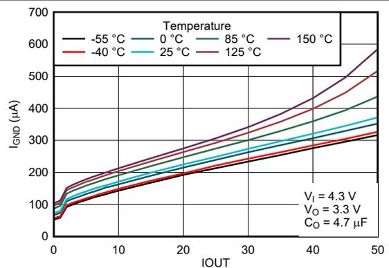
图 6-18. Ground Pin Current vs Load Current for New Chip
