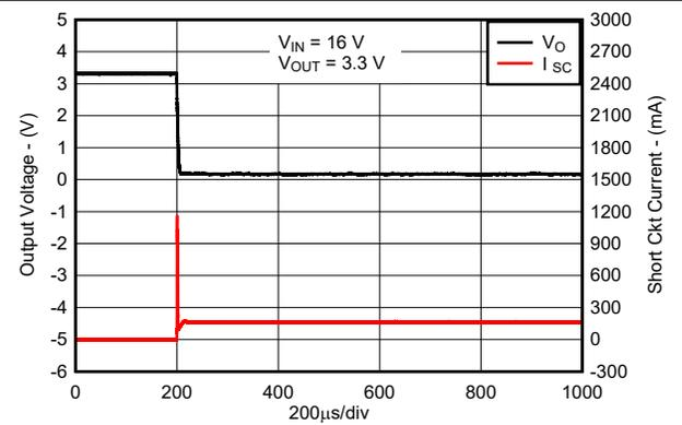
图 6-24. Short-Circuit Current vs Time for New Chip
