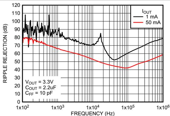
$V_{OUT} = 3.3\text{ V}$ ,  $C_{OUT} = 2.2\ \mu\text{F}$ ,  $C_{FF} = 10\text{ pF}$
