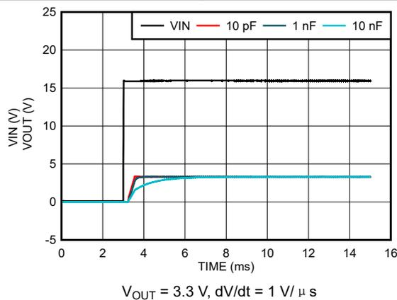
图 8-7. Start-Up vs  $C_{FF}$  for New Chip
