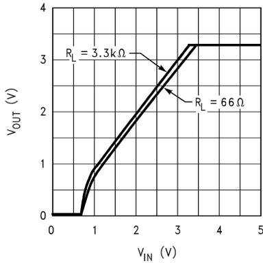
图 6-3. Output Voltage vs  $V_{IN}$  for Legacy Chip
