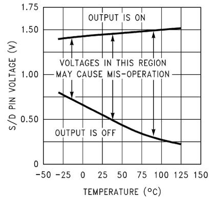
图 6-32. ON/OFF Threshold vs Temperature for Legacy Chip
