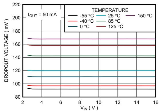
图 6-6. Dropout Voltage vs  $V_{IN}$  and Temperature for New Chip
