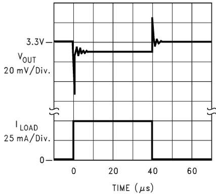
图 8-3. Load Transient Response for Legacy Chip
