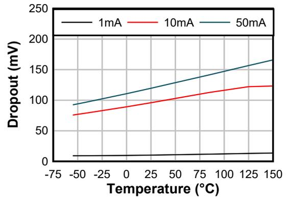
图 6-8. Dropout Voltage vs Temperature for New Chip
