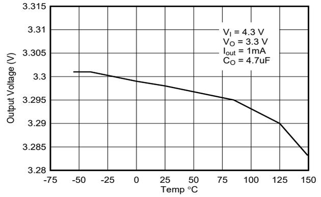
图 6-2. Output Voltage vs Temperature for New Chip
