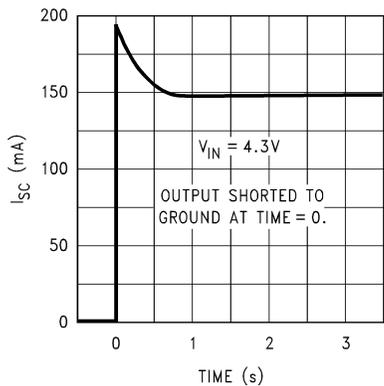
图 6-21. Short-Circuit Current vs Time for Legacy Chip
