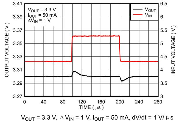
图 8-6. Line Transient Response for New Chip
