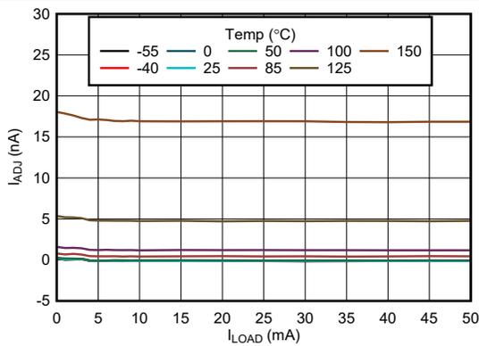
图 6-29. ADJ Pin Bias Current vs Load Current for New Chip
