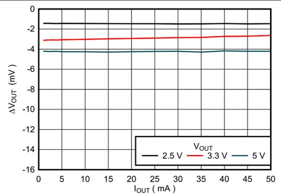
图 6-12. Output Regulation vs Load Current for New Chip
