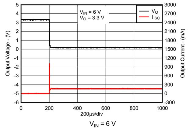
图 6-22. Short-Circuit Current vs Time for New Chip
