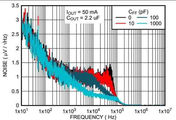
$V_{IN} = 4.3\text{ V}$ ,  $V_{OUT} = 3.3\text{ V}$ ,  $I_{OUT} = 50\text{ mA}$ ,  $C_{OUT} = 2.2\text{ }\mu\text{F}$
