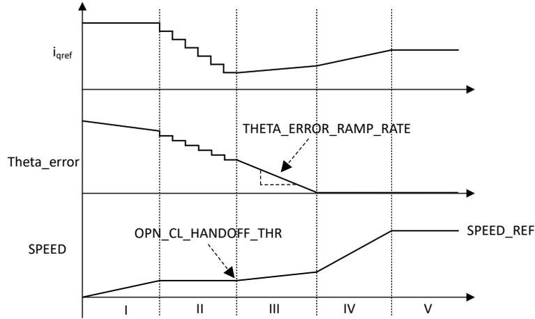
I. Open Loop Acceleration, II. Current Decay, III. Closed loop slow acceleration
