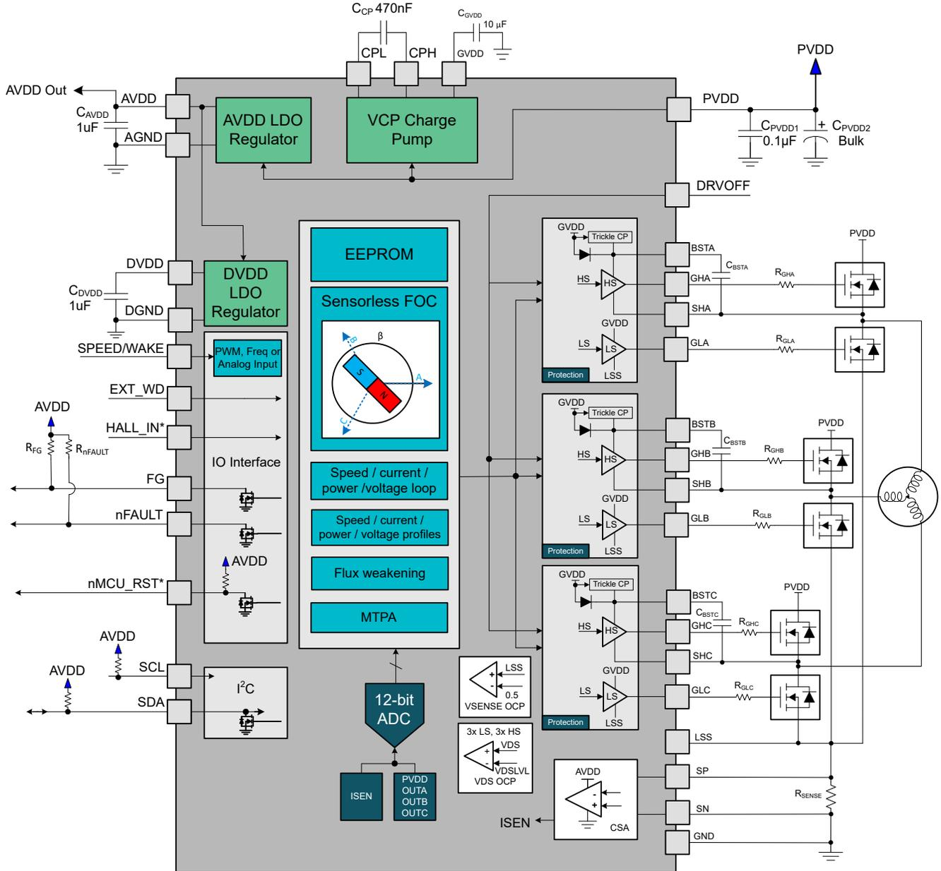
\*HALL\_IN and nMCU\_RST are mux'ed functions on pin 30
