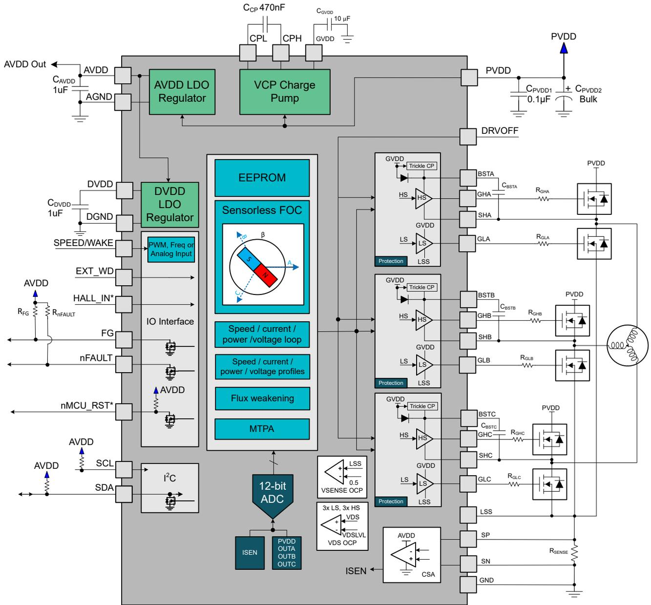
\*HALL\_IN and nMCU\_RST are mux'ed functions on pin 30
