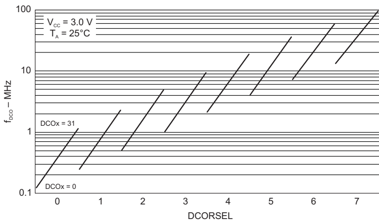
Figure 5-10. Typical DCO Frequency
