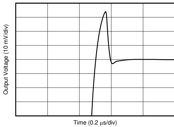
D032 V_S = 5.5\text{ V} V_{\text{ICM}} = 2.75\text{ V} V_{\text{OCM}} = 2.75\text{ V} C_L = 0 Gain = 1 5-V step
