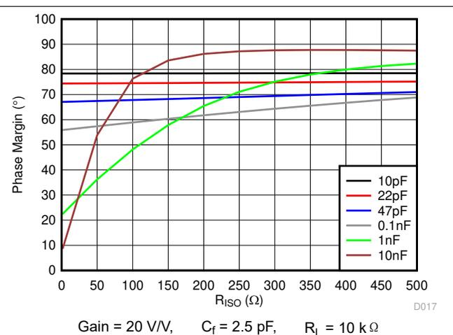
**图 8-3. Phase Margin vs. Series Isolation Resistor**
