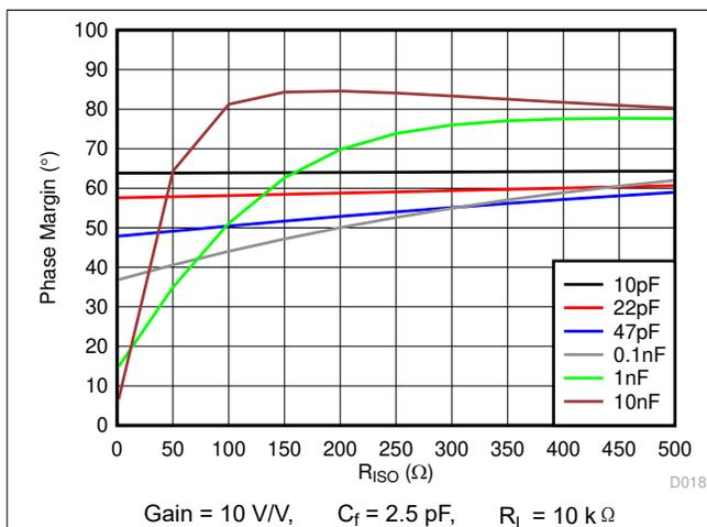
**图 8-2. Phase Margin vs. Series Isolation Resistor**
