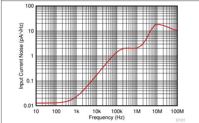
图 7-3. Input Current Noise Density vs Frequency
