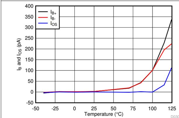
图 7-29. Input Bias and Offset Current vs Temperature
