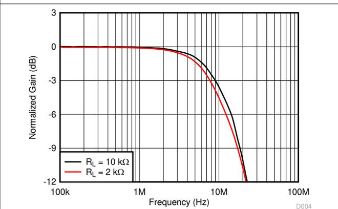
图 7-6. Small-Signal Frequency Response vs Output Load
