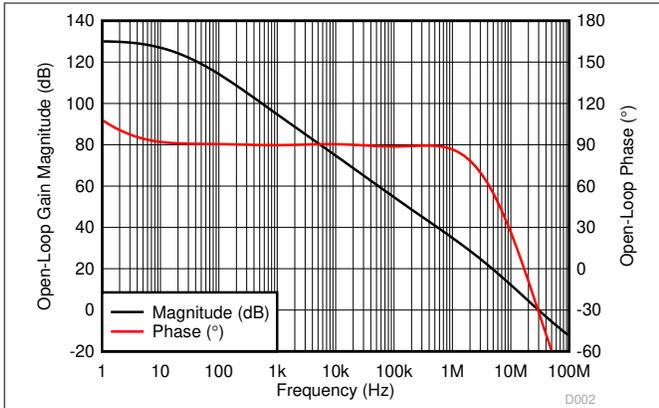
图 7-1. Open Loop Gain and Phase vs Frequency
