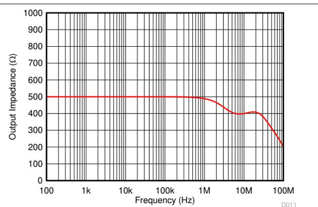
图 7-12. Open Loop Output Impedance vs Frequency
