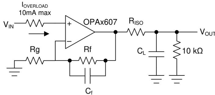
**图 8-1. Input Current Protection and Driving Capacitive Loads**
