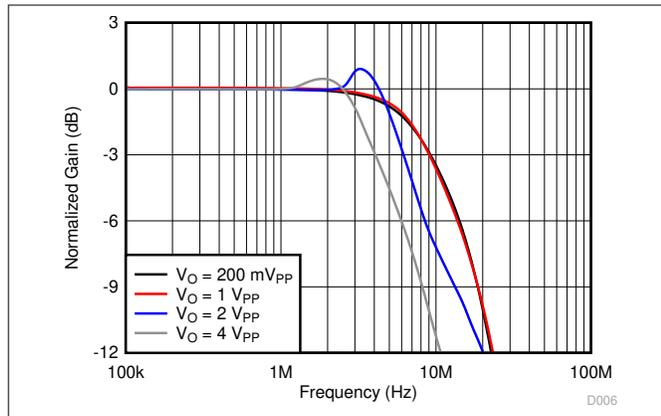
图 7-7. Large-Signal Frequency Response vs Output Voltage
