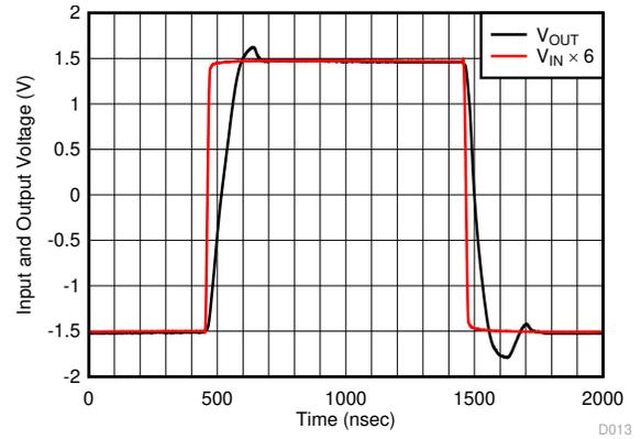
$T_{RISE} = 1\ \mu\text{sec}$ ,  $T_{FALL} = 0.7\ \mu\text{sec}$
