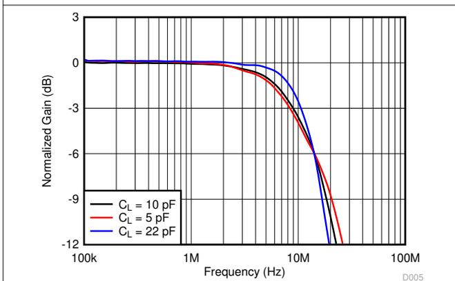
图 7-5. Small-Signal Frequency Response vs Capacitive Load
