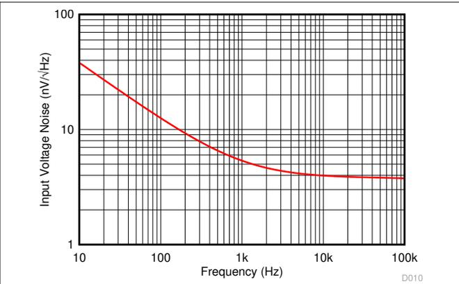
图 7-2. Input Voltage Noise Density vs Frequency
