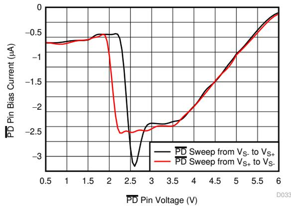
图 7-21. Power Down Pin Bias Current vs Power Down Pin Voltage
