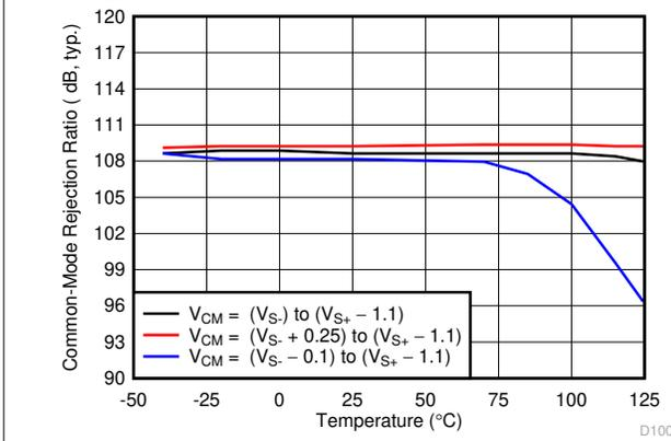
图 7-27. Common Mode Rejection Ratio vs Temperature
