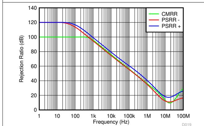
图 7-11. Rejection Ratio vs frequency
