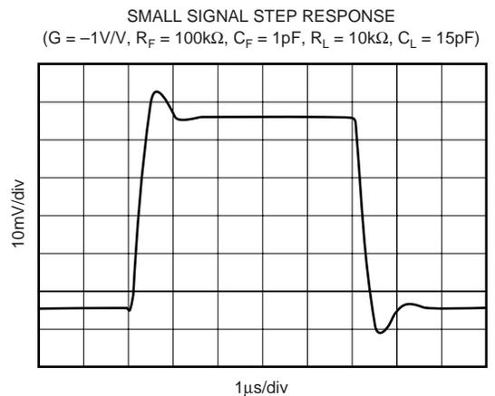
NOTE:  $C_F$  is used to optimize settling time.
