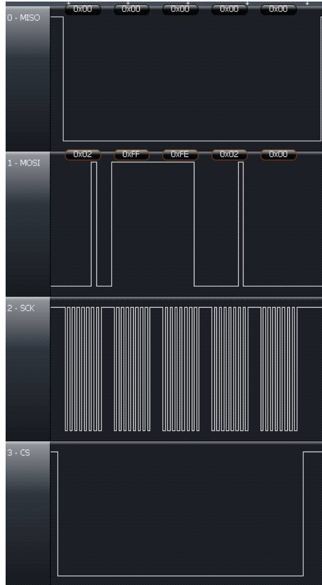
图 5-8. SPI Access Example: Write of the Control Register at Address 0xFFFE With 0x00, 0x02 (RF Enable = 1)
