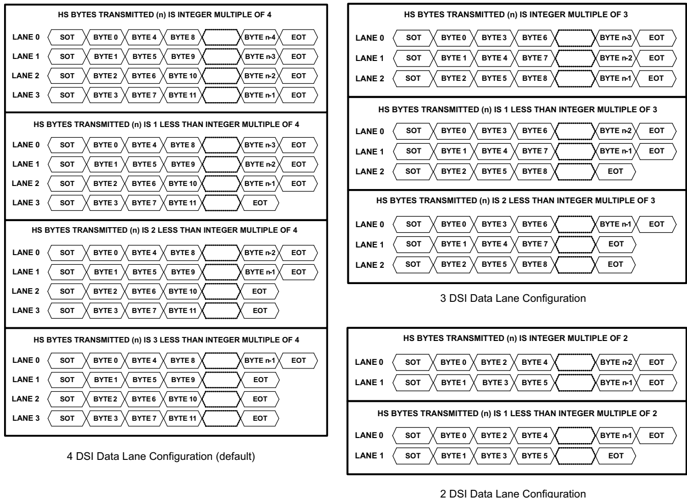
Figure 13. SN65DSI83-Q1 DSI Lane Merging Illustration
