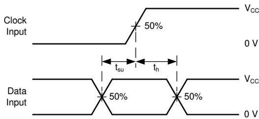
图 7-3. Voltage Waveforms, Setup and Hold Times
