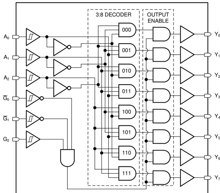
图 8-1. Logic Diagram (Positive Logic) for SN74HCS238
