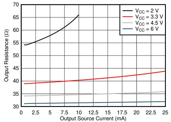
图 6-2. Output driver resistance in HIGH state.
