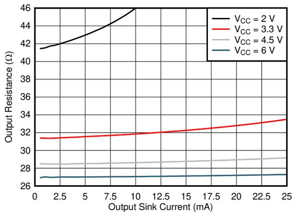
图 6-1. Output driver resistance in LOW state.
