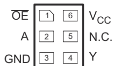
图 5-1. DBV package 5-pin SOT-23 (Top View)
