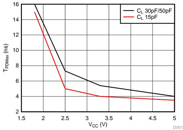
**Figure 1. Propagation delay vs V<sub>CC</sub>**
