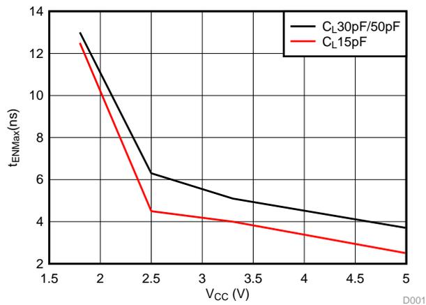
**Figure 7. Enable Time vs V<sub>CC</sub>**
